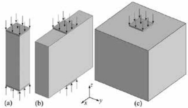
Fig. 1: Illustrations of: (a) rectangular prismatic strut; (b) 2-D rectangular bottle-shaped strut; and (c) 3-D rectangular bottle-shaped strut (after Laughery and Pujol<sup>4</sup>)
