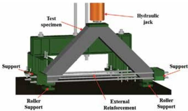
**Fig. 4:** Schematic of test setup and specimen with supports (truss-like specimen shown)
