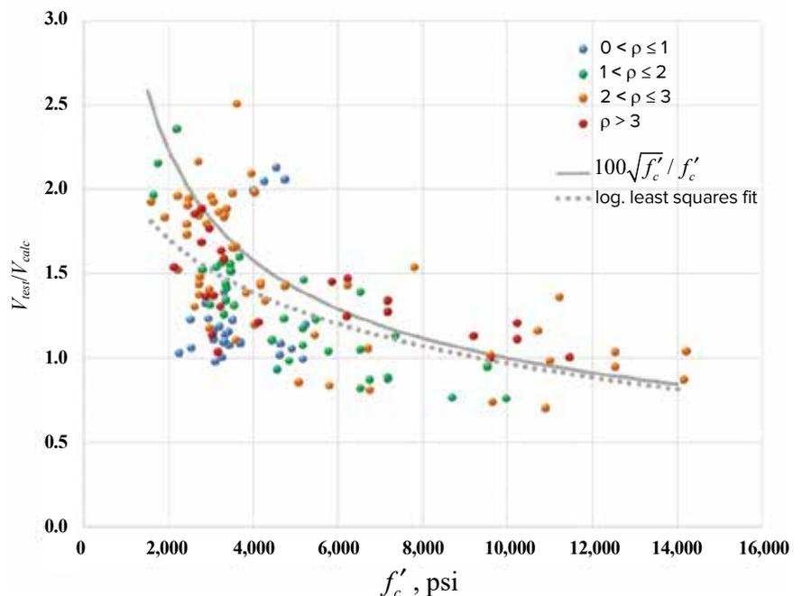
Fig. 3:  $V_{test}/V_{calc}$  versus  $f'_c$  (Note:  $V_{calc}$  in accordance with the strut-and-tie method in ACI 318-14;  $\rho$  = longitudinal reinforcement ratio, %)
