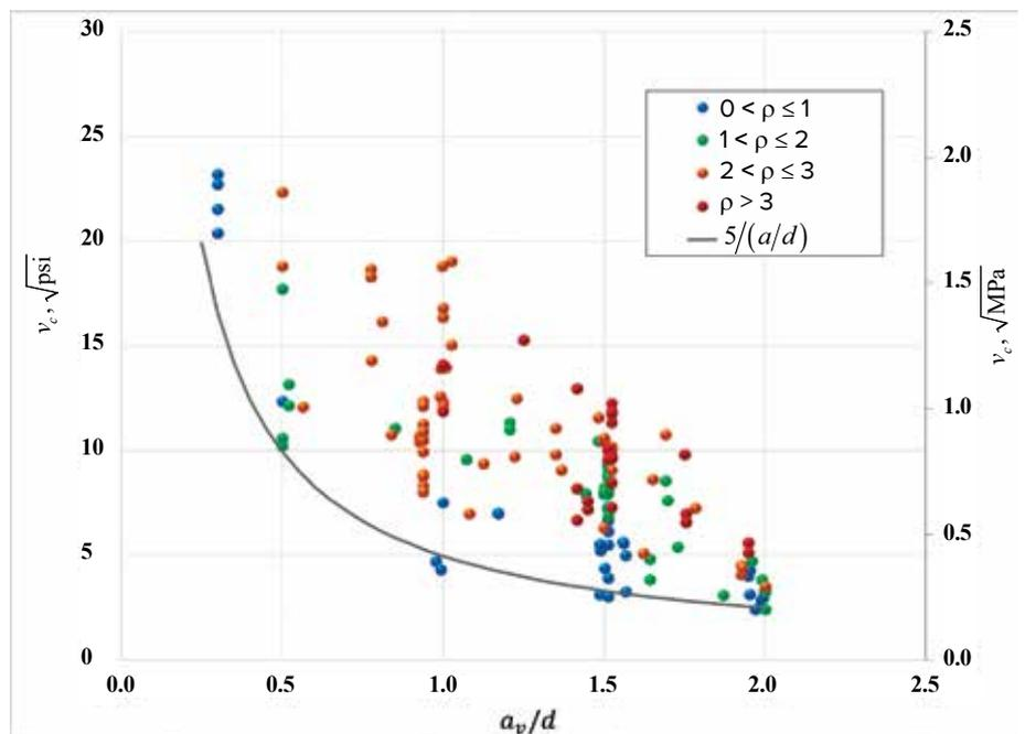
Fig. 7: Shear stress  $v_c$  versus ratio of shear span to effective depth,  $a_v/d$  (Note:  $v_c = V_{test}/bd$ )
