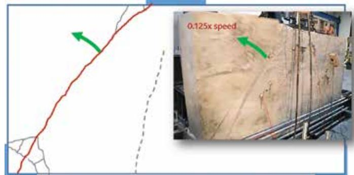
**Fig. 5:** Failure crack pattern and image of instant of failure for specimen Re-45-Ex
