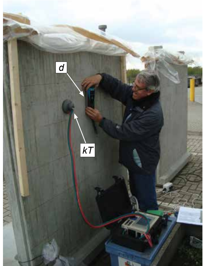
Fig. 5: Measuring kT and d on site
