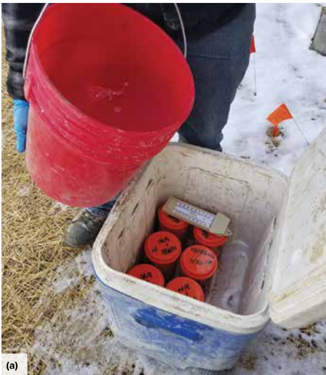
Fig. 4: Example of curing in a beverage cooler: (a) a technician adds water to submerge specimens in covered molds; and (b) the cooler is marked to help mitigate disturbance during initial curing
