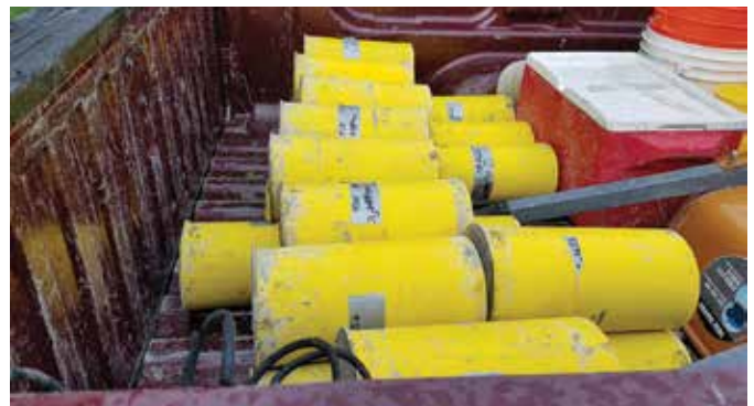
Fig. 1: Example of improper transportation of test specimens. Early-age specimens are fragile and susceptible to mechanical damage if not protected from jarring. In this example, the specimens are not restrained and can be affected by impact with each other and other surfaces. Lastly, the specimen molds lack covers for controlling moisture loss
