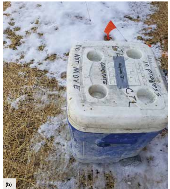
Fig. 4: Example of curing in a beverage cooler: (a) a technician adds water to submerge specimens in covered molds; and (b) the cooler is marked to help mitigate disturbance during initial curing
