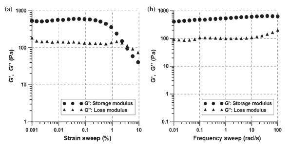
Fig. 4 Representative results of dynamic oscillatory shear measurement. a Strain sweep, b Frequency sweep.
