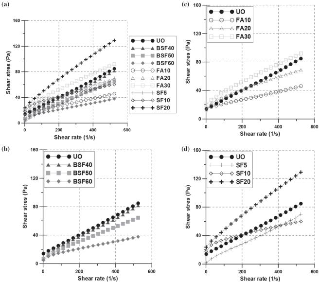
Fig. 3 Results of steady shear measurement. a All cases, b UO and BSF cases, c UO and FA cases, d UO and SF cases.
