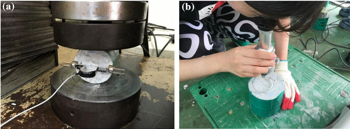
**Fig. 1** Photographs for crack inducing and crack measurement. **a** Crack inducing and gauge setup. **b** Crack width measurement.
