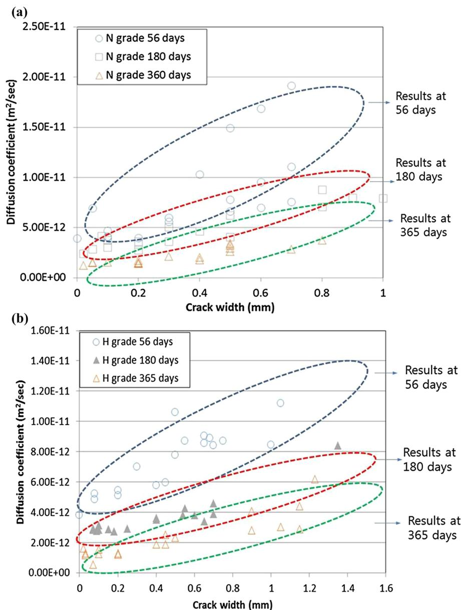
**Fig. 4** Changes in diffusion coefficient under steady state condition with various crack width. **a** Enlarged diffusion coefficient in cracked concrete (N grade). **b** Enlarged diffusion coefficient in cracked concrete (H grade).
