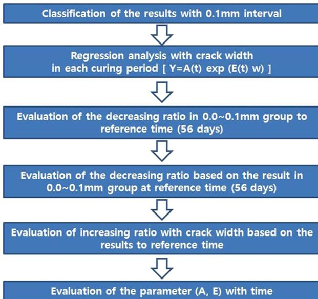
**Fig. 5** Flowchart for quantification of crack and age effect on diffusion.
