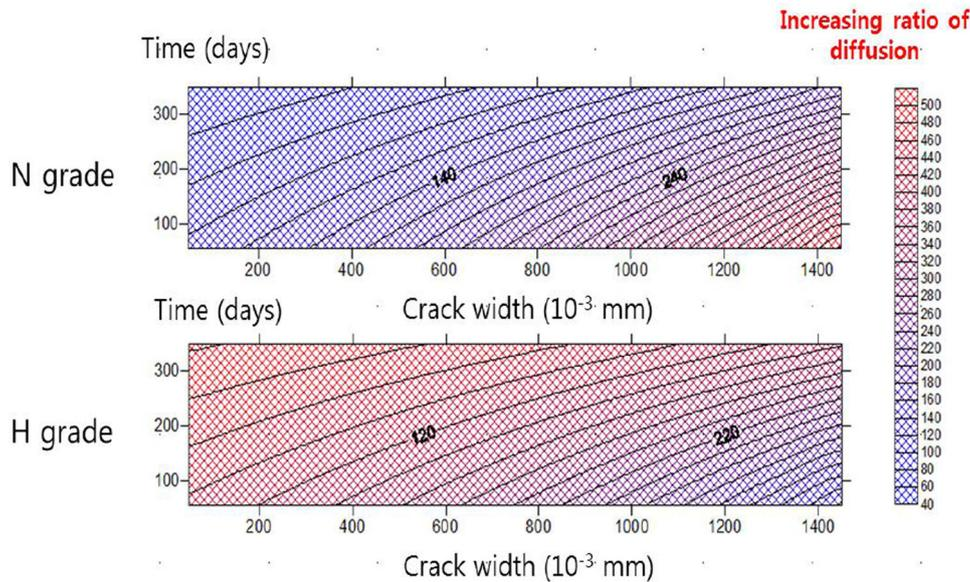
Fig. 9 Diffusion coefficient contours with time and age effect.
