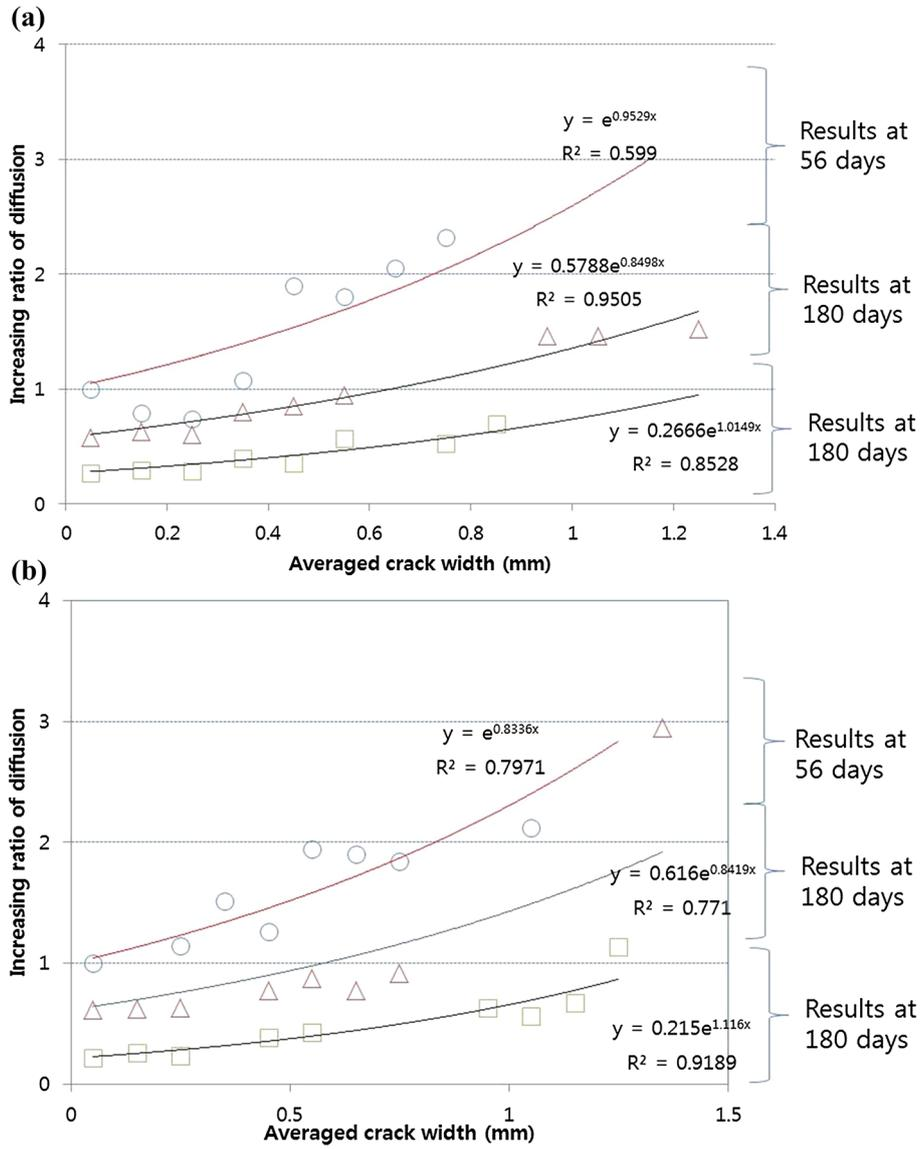
**Fig. 6** Diffusion normalization with time and crack width. **a** Result normalization of N grade. **b** Result normalization of H grade.
