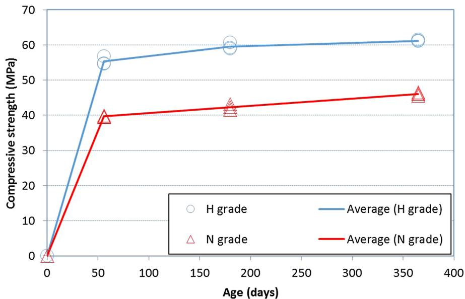
**Fig. 3** Changes in compressive strength with different curing ages.
