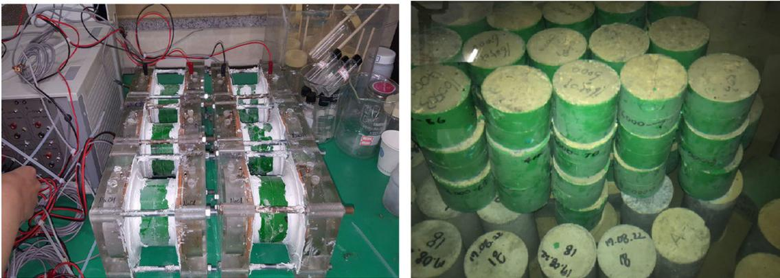
**Fig. 2** Photographs of accelerated diffusion test setup and concrete samples under curing.
