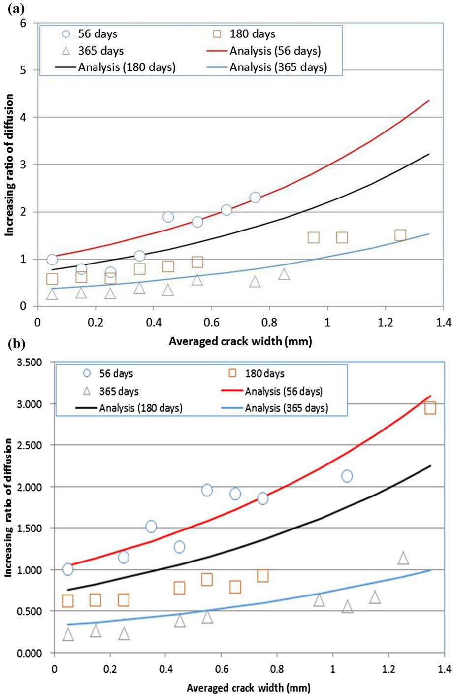
Fig. 8 Diffusion coefficient of test and regression analysis. a N-grade. b H-grade.
