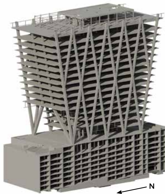
Fig. 1: The building structure features a unique lateral system consisting of a diagonalized, architecturally exposed concrete exoskeleton
