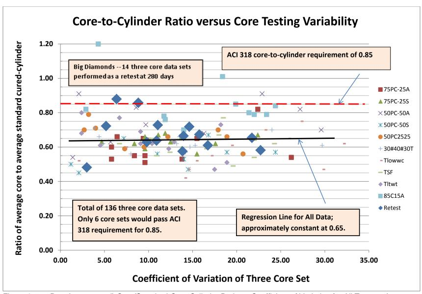
Figure 3.5 Raw (uncorrected) Core/Standard-Cure Cylinder Ratio vs Coefficient of Variation for All Tests at Ages Ranging from 28 to 280 days.
