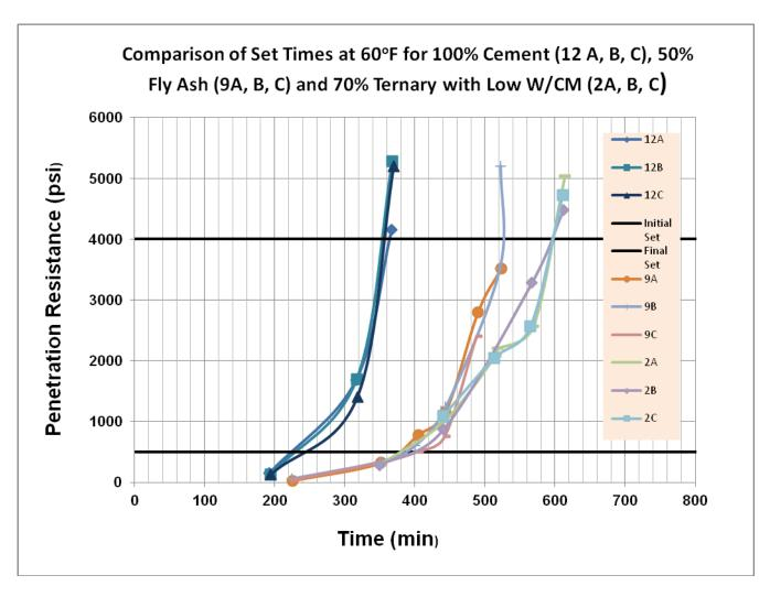
Figure 5.4 Penetration resistance versus time for three different mixtures at 60°F: 100% portland cement, 50% fly ash and 70% ternary with low water-cementitious ratio. Note that the use of SCM's significantly delayed setting.
