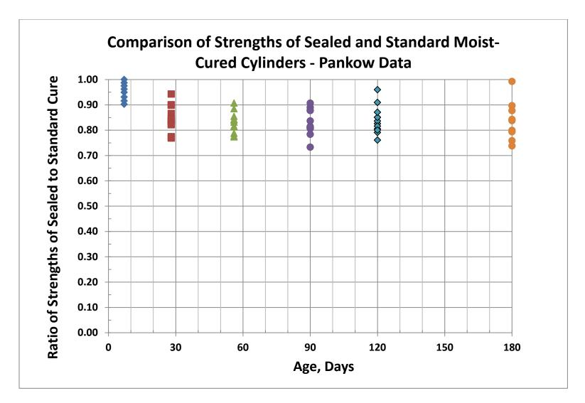
Figure 2.2 Pankow Data: Sealed-cure to water-cure strength ratios for cylinders at ages up to 180 days
