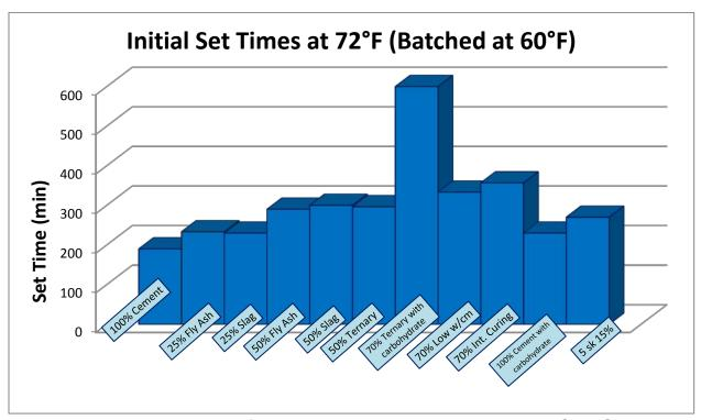
Figure 5.3 Initial setting times for concrete mixtures as measured by ASTM C 403. Initial setting times vary from a low of 190 minutes for the 100% cement mixture to greater than 780 minutes for the 70% ternary mixture with a carbohydrate-based admixture. Note that the carbohydrate-based admixture did not substantially increase initial setting time when used with the 100% cement mixture. All other concrete mixtures contained a polycarboxylate water-reducing admixture.
