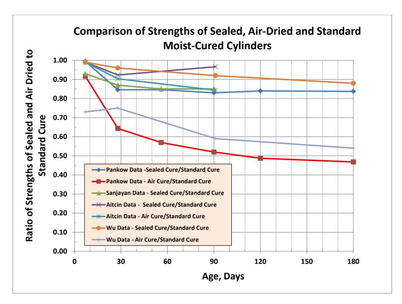
Figure 2.3 Average sealed-cure to water-cure and air-cure to water-cure strength ratios for cylinders at ages up to 180 days.
