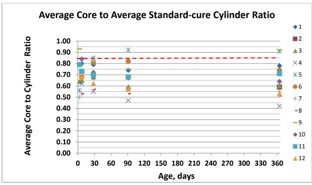
Figure 3.4 Average same-age core-to-cylinder ratios for Bloem's 1968 well-cured slabs. Note that very few results show a core-to-cylinder ratio above 0.85.
