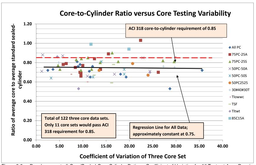
Figure 3.6 Raw (uncorrected) Core/Sealed-Cure Cylinder Ratio vs Coefficient of Variation for All Tests at Ages Ranging from 28 to 180 days.
