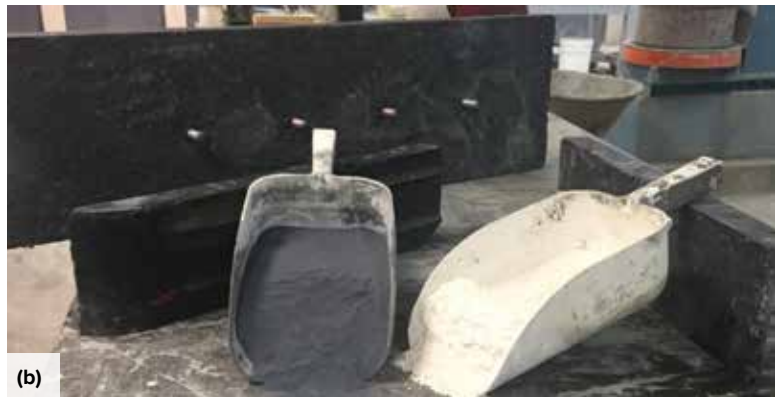
Fig. 6: Concrete runners: (a) formwork and stainless steel attachments; and (b) finished runners (without external GFRP wrap)
