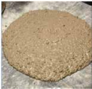
Fig. 2: Slump flow of the self-consolidating GP control mixture
