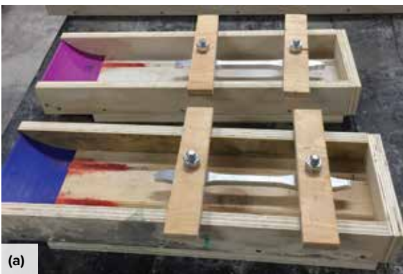
Fig. 6: Concrete runners: (a) formwork and stainless steel attachments; and (b) finished runners (without external GFRP wrap)
