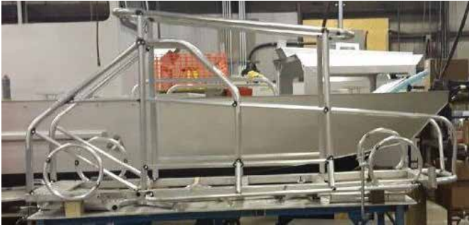
Fig. 1: The toboggan framework was designed to safely carry five riders
