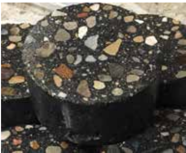
Fig. 5: Cross section of a 28-day SF50 concrete cylinder
