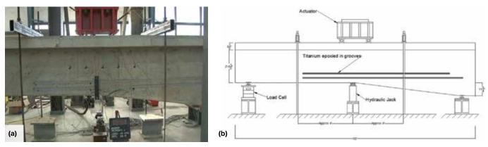
Fig. 3: Full-scale beam testing was used to verify the adequacy of the proposed repairs for the Mosier bridge: (a) photo of a strengthened beam prior to testing; and (b) schematic of test apparatus (Note: 1 ft = 0.30 m; 1 in. = 25 mm) (photo and schematic courtesy of Christopher Higgins, OSU)
