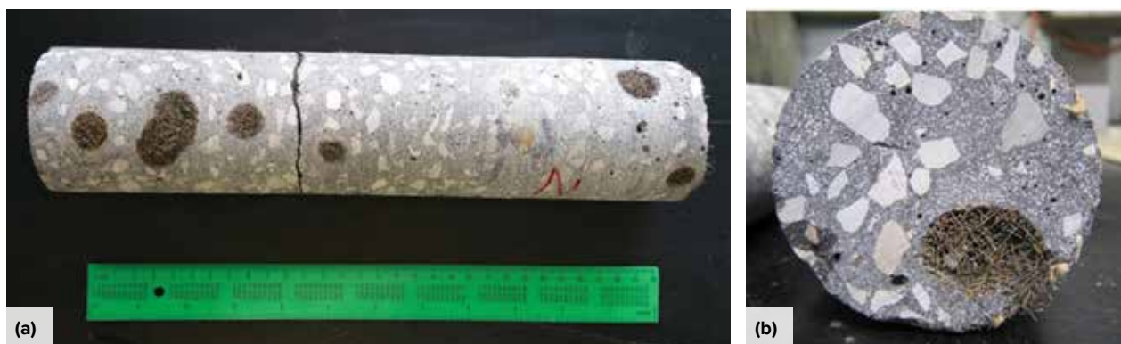
Fig. 2: UHPC core taken from a large UHPC placement in which mixing was performed in a concrete truck: (a) view of the circumference; and (b) a cross section with a fiber ball
