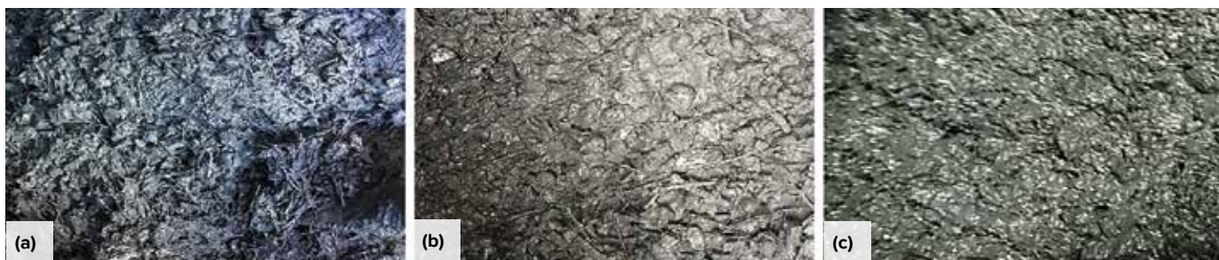
Fig. 6: The appearance of the fresh UHPC mixture in a drum mixer when: (a) 50% of fine steel fibers are replaced with steel hooked fibers; (b) 50% of fine steel fibers are replaced with medium-sized steel fibers; and (c) 25% of fine steel fibers are replaced with medium-sized steel fibers
