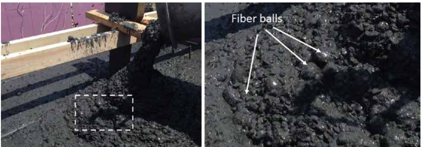
Fig. 1: Fiber balls observed in a large-scale UHPC batch produced in a concrete truck
