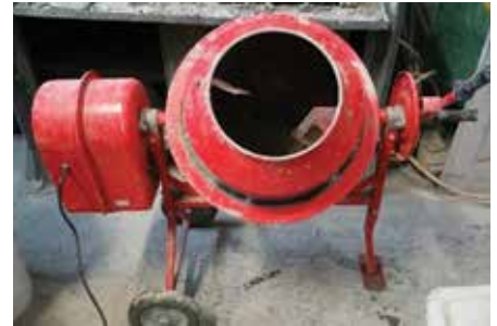
Fig. 4: The laboratory-scale rotary drum mixer used in this investigation
