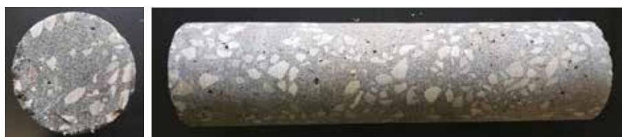
Fig. 7: Pictures of a core extracted from a UHPC placement prepared in a concrete truck where 50% of fine steel fibers was replaced with medium-sized steel fibers
