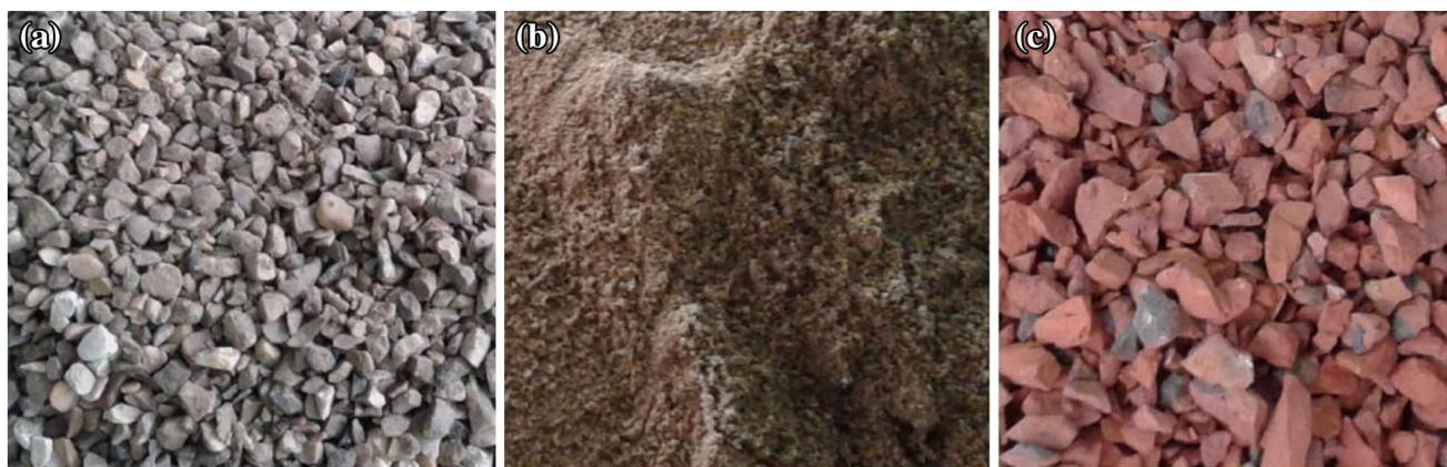
**Fig. 1** Aggregates (a) stone chips (b) sand (c) masonry chip aggregate (MCA).
