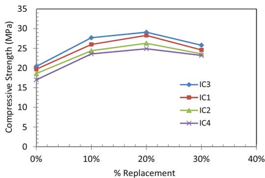
**Fig. 6** Effect of percent replacement on compressive strength of control and internally cured samples with w/c ratio of 0.4 under similar curing conditions (Phase I).
