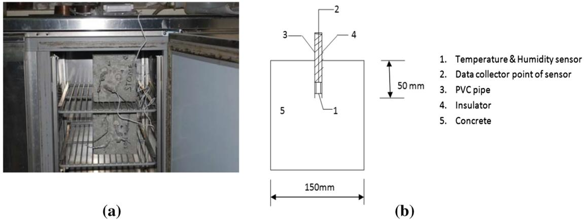
Fig. 10 Internal RH measurement a experimental diagram b schematic diagram.
