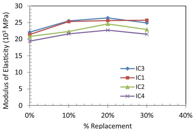
**Fig. 8** Effect of percent replacement on modulus of elasticity of control and internally cured samples with w/c ratio of 0.4 under similar curing conditions.
