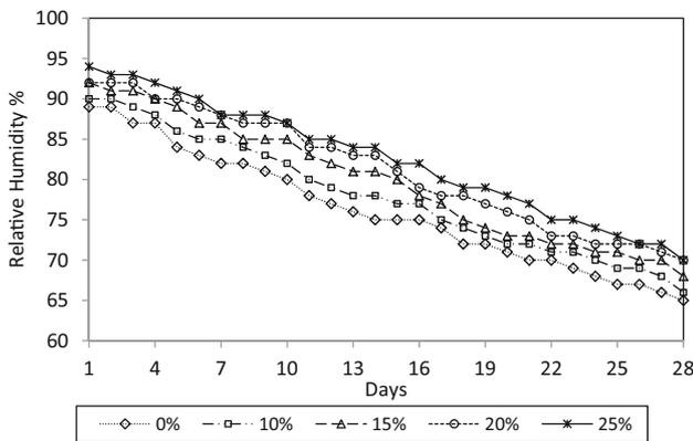
Fig. 11 Internal RH data of control samples and internally cured samples with respect to days.
