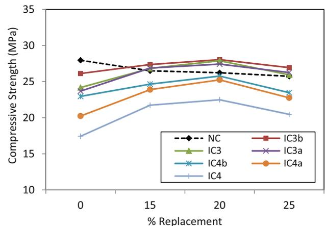
Fig. 12 Effect of percent replacement on compressive strength (Phase II).
