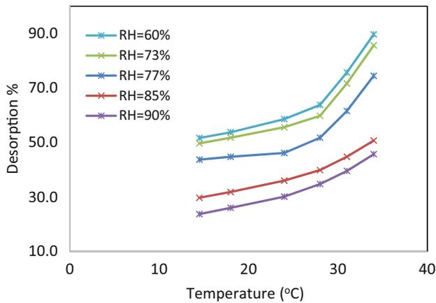
**Fig. 3** Effect of temperature on desorption rate of MCA.
