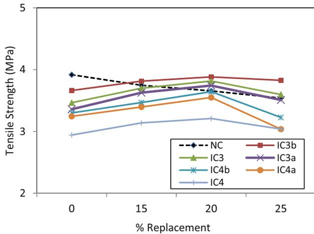
**Fig. 13** Effect of percent replacement on splitting tensile strength (Phase II).
