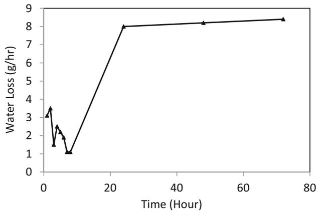
**Fig. 4** Effect of time on desorption rate of MCA for a constant temperature (34 °C) and constant relative humidity (73%).
