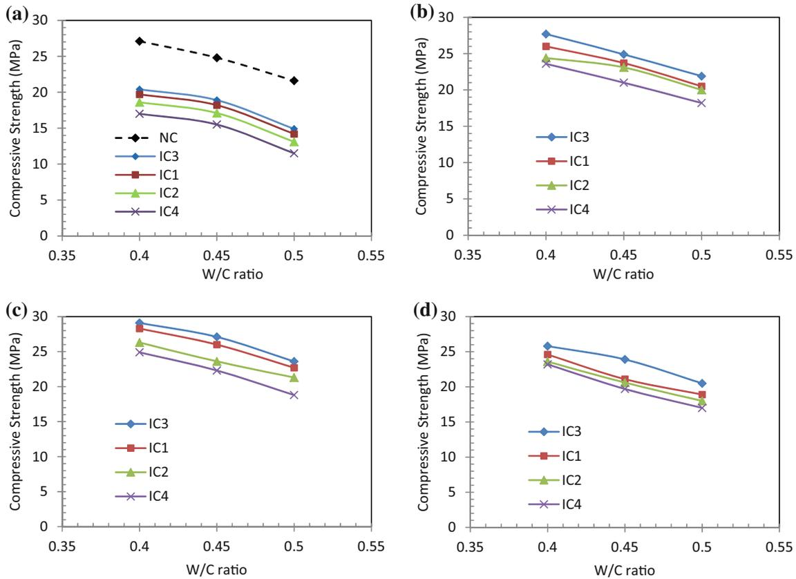
**Fig. 5** Effect of w/c ratio on 28 day compressive strength of samples **a** control samples with 0% replacement **b** IC samples with 10% replacement **c** IC samples with 20% replacement **d** IC samples with 30% replacement.
