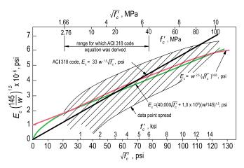
Fig. 1: Secant modulus of elasticity versus concrete strength, based on Reference 3
