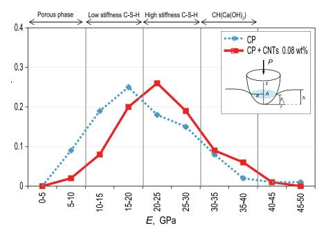
Fig. 10: Probability plots of the MOE for 28-day cement paste (w/cm = 0.485) and cement paste reinforced with 0.08% CNTs by weight of cement<sup>11</sup> (Note: 1 GPa = 145,000 psi)
