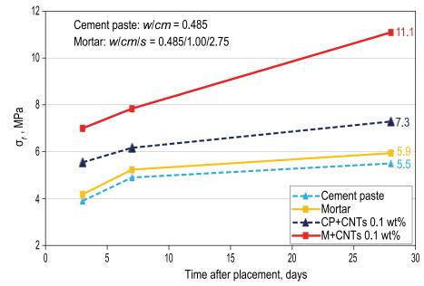
Fig. 5: Rate of development of flexural strength  $\sigma_r$  of the control cement paste (CP) and mortar (M) specimens and cement pastes and mortars reinforced with 0.1% CNTs by weight of cement (based on References 14 and 15) (Note: 1 MPa = 145 psi)
