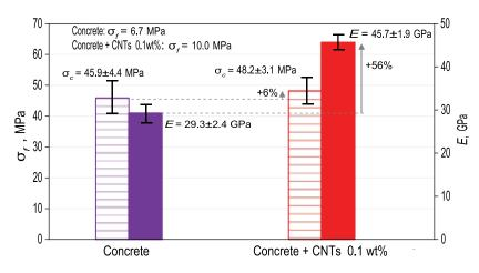
Fig. 9: Compressive strength at 28 days,  $\sigma_c$ , and MOE for concrete and concrete reinforced with 0.1% CNTs by weight of cement (Note: 1 MPa = 145 psi; 1 GPa = 145,000 psi)
