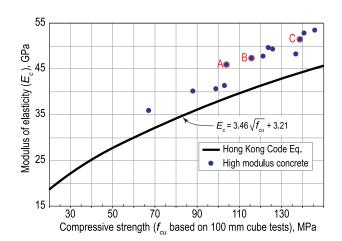
Fig. 2: Compressive strength versus modulus of elasticity (based on References 4 and 5). Mixture proportions for A, B, and C are listed in Table 1 (Note: 1 GPa = 145,000 psi; 100 mm = 4 in.; 1 MPa = 145 psi)
