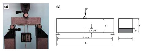
Fig. 6: Notched specimen tests: (a) three-point bending test setup with gauge used to measure crack mouth opening displacement (CMOD); and (b) geometry of notched specimens<sup>16</sup>
