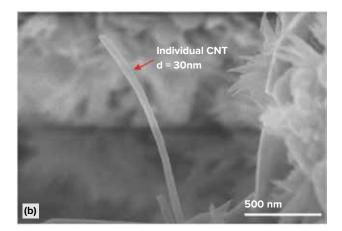
Fig. 4: SEM image of cement paste nanocomposites reinforced with CNTs: (a) produced without ultrasonication procedure; and (b) produced using an HRWRA (surfactant) and ultrasonic energy<sup>10</sup>
