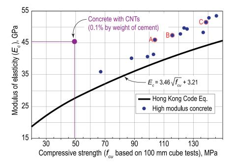
Fig. 11: Updated version of Fig. 2, showing the increase in MOE due to using CNTs in concrete (Note: 1 GPa = 145,000 psi; 100 mm = 4 in.; 1 MPa = 145 psi)
