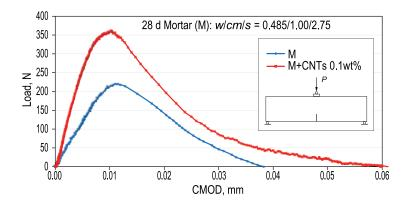
Fig. 8: Crack mouth opening displacement (CMOD) versus load (at 28 days) for notched beam specimens fabricated from mortar (M) and mortar reinforced with 0.1% CNTs by weight of cement<sup>15</sup> (Note: 1 N = 0.225 lbf; 1 mm = 0.04 in.)
