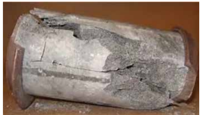
A compression test specimen. Is this failure mode acceptable? Is there evidence of preparation errors that would impact the test result? A certified CQTM is expected to know the answers
