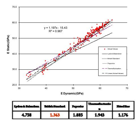
**Figure 10.** Comparison of E (ASTM C469) vs.  $E_d$  (ASTM C215) data (points) using longitudinal resonance for concrete cylinders. Various relations between E and  $E_d$  are also shown as lines. The mean absolute error (in GPA) for each type of fit curve is shown in the table underneath. Data obtained from CTLGroup.
