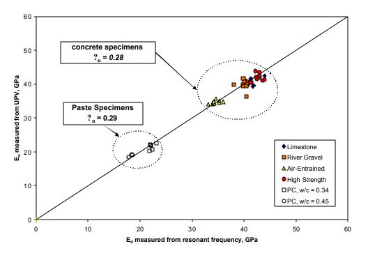
**Figure 7.** Comparison of  $E_d$  values obtained by longitudinal resonance frequency (ASTM C215) and ultrasonic pulse velocity (ASTM C597) tests carried out on concrete and paste cylinders. Unusually high values of Possion's ratio were assumed for the predictions based on pulse velocity.
