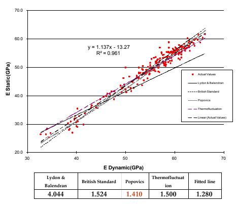
**Figure 11.** Comparison of E (ASTM C469) vs.  $E_d$  (ASTM C215 using transverse resonance) data (points) for concrete cylinders. Various relations between E and  $E_d$  are also shown as lines. The mean absolute error (in GPA) for each type of fit curve is shown in the table underneath. Data obtained from CTLGroup.
