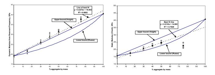
**Figure 9.** Variation of dynamic (left) and static (right) Young's modulus as a function of aggregate content in the two-phase composite concrete specimens. Ed determined using longitudinal resonance following the ASTM C215 procedure.
