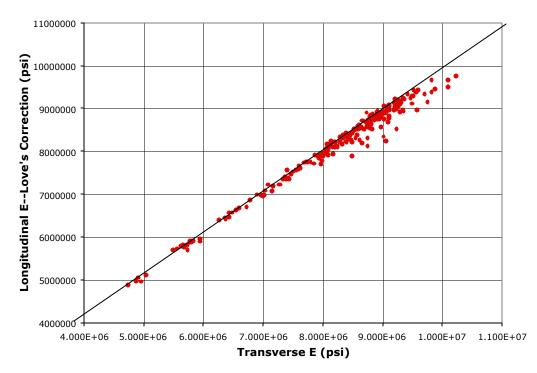
**Figure 5.** Comparison of longitudinal and transverse  $E_d$  values. Longitudinal values obtained using Love's correction (assumed v = 0.25) and transverse values obtained using ASTM C215 method on concrete cylinders. Test data provided by CTLGroup.
