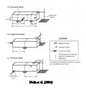
Figure 2. Testing configuration for standard vibrational resonance tests (Naik et a. 2004)
