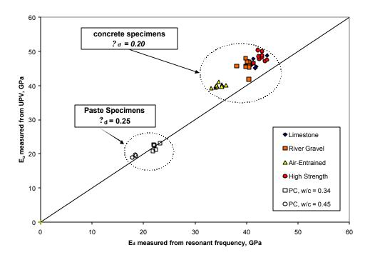
**Figure 6.** Comparison of  $E_d$  values obtained by longitudinal resonance frequency (ASTM C215) and ultrasonic pulse velocity (ASTM C597) tests carried out on concrete and paste cylinders. Median values of Possion's ratio were assumed for the predictions based on pulse velocity.
