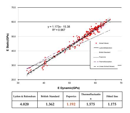
**Figure 12.** Comparison of E (ASTM C469) vs.  $E_d$  (Love's correction using longitudinal resonance) data (points) for concrete cylinders. Various relations between E and  $E_d$  are also shown as lines. The mean absolute error (in GPA) for each type of fit curve is shown in the table underneath. Data obtained from CTLGroup.
