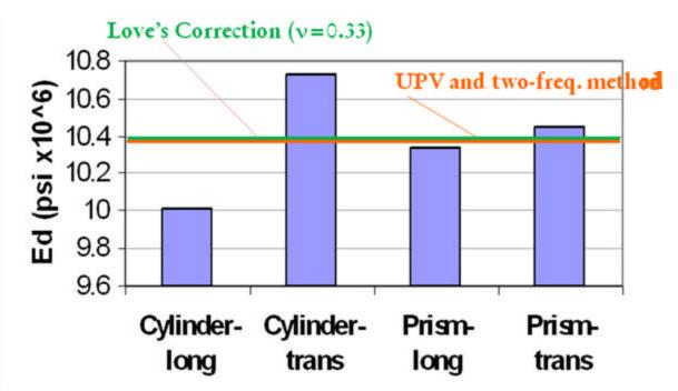
**Figure 3.** Comparison of longitudinal and transverse  $E_d$  values obtained using ASTM C215 method on aluminum samples. The expected E value is  $10.4 \times 10^6$  psi and v is 0.33.
