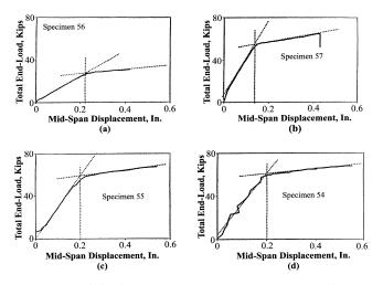
*Fig.* 7—Load-displacement response of specimens with stirrups: (a) Specimen 56; (b) Specimen 57; (c) Specimen 55; and (d) Specimen 54.
