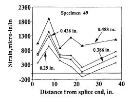
Fig. 11—Strain in stirrups placed over splice region: Specimen 49.
