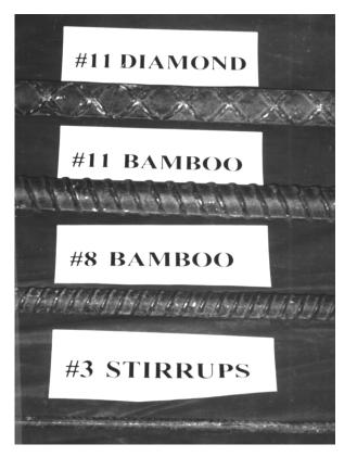
Fig. 2—Different bar sizes used in experimental program.
