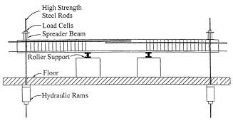
Fig. 3—Test setup.
