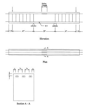
Fig. 1—Test specimen.
