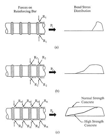
Fig. 4—Freebody diagram of reinforcing bar embedded in concrete and subjected to tension.
