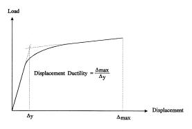
Fig. 6—Definition of displacement-ductility ratio.
