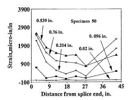
Fig. 10—Strain in stirrups placed over splice region: Specimen 50.
