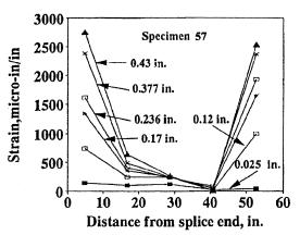
Fig. 9—Strain in stirrups placed over splice region: Specimen 57.
