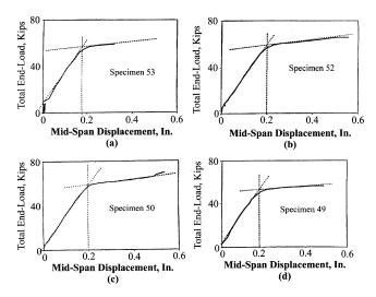
Fig. 8—Load-displacement response of specimens with stirrups: (a) Specimen 53; (b) Specimen 52; (c) Specimen 50; and (d) Specimen 49.
