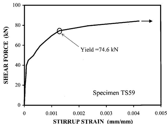
Fig. 4—Load-stirrup strain curve for TS59.
