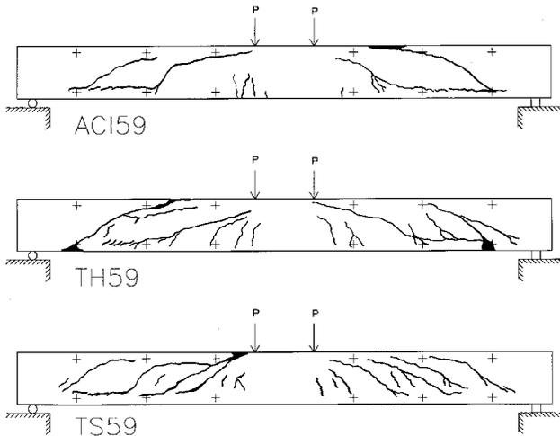
Fig. 5—Crack pattern; beams of Series 59.
