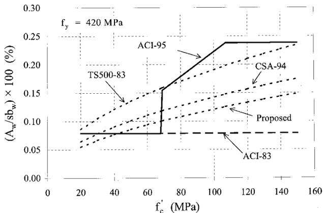
Fig. 1—Comparison of minimum shear reinforcement requirements to ACI 318-83, TS500-83, and the proposed equation, test results could also be used to evaluate CSA A23.3-94 and ACI 318-95 requirements.
