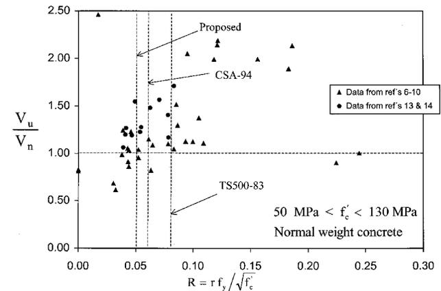
Fig. 11—Variation of  $V_u/V_n$  with shear reinforcement index.
