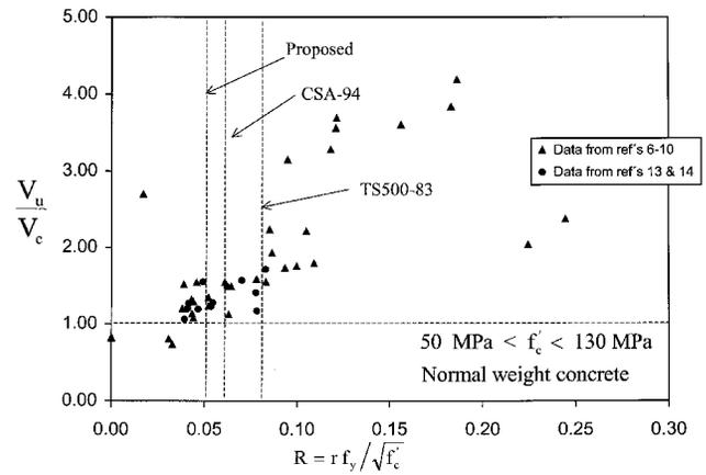
Fig. 10—Variation of  $V_u/V_c$  with shear reinforcement index.
