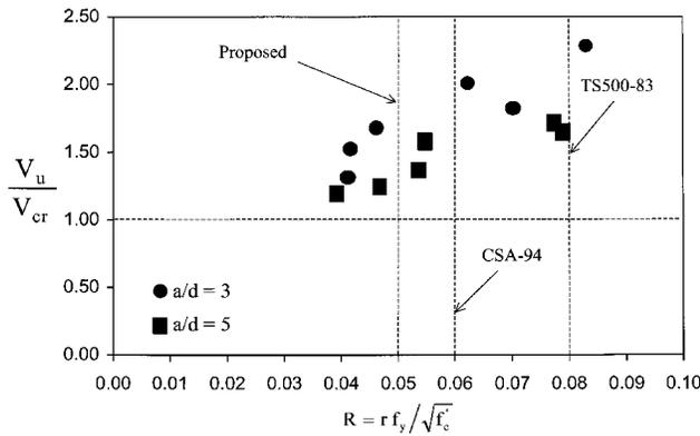
Fig. 9—Variation of  $V_u/V_{cr}$  with shear reinforcement index.
