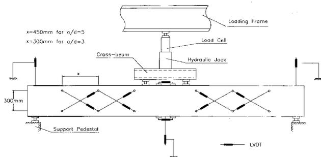
Fig. 3—Test setup and instrumentation (external).
