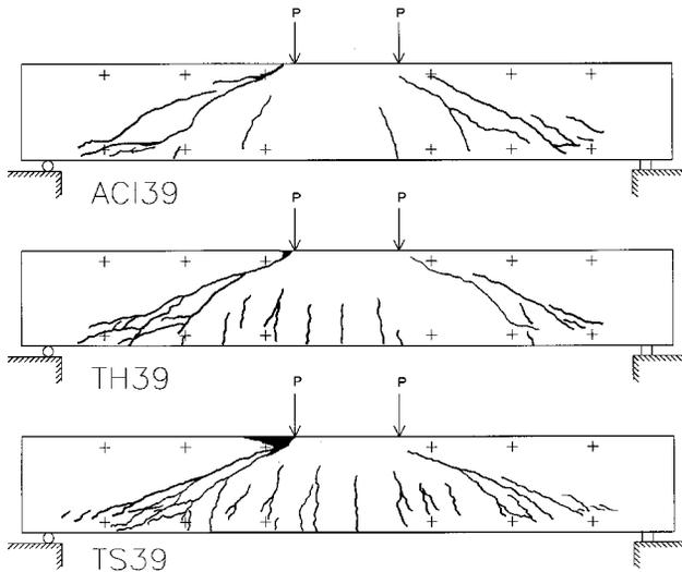
Fig. 7—Crack pattern: beams of Series 39.
