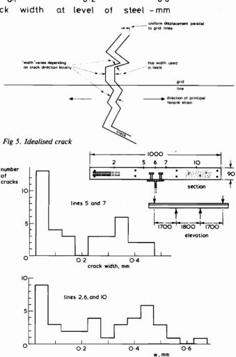
Fig 6. Crack widths in beam UC6, load stage 9
