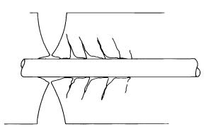
b internal cracking & concrete deformation
