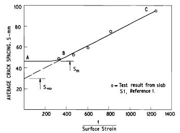
Fig 10. Plot of crack spacing against surface strain
