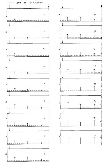
Fig 2. Sequence of cracking of the first flexural cracks at 11.70 kN (cracking load)
