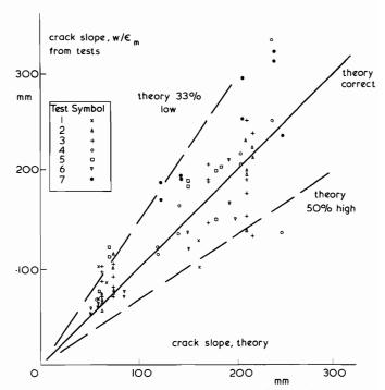
Fig 7. Crack widths in seven composite beams under negative moment, compared with prediction by the C & CA method (Report 42.468, June 1972) for members in pure tension
