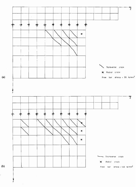
Fig 1. Formation and propagation of internal cracks in reinforced concrete tension specimens
