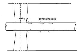
a slip & concrete deformation
