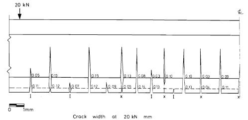
Fig 3. Crack width at 20 kN mm
