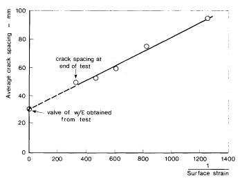
Fig 9. Relationship between crack spacing and surface strain (specimen SI)
