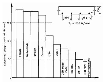
Fig 1. Design crack widths calculated using various regulations for the slab shown
