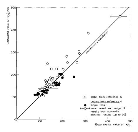
Fig. 8. Comparison of experimental and calculated values of crack width/strain  $(w/\epsilon)$  with a 5% chance of exceedence
