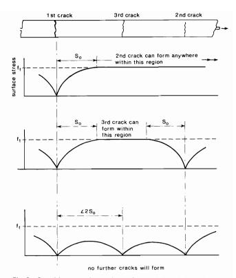
Fig 2. Conditions on the surface of an axially reinforced tension member during the development of cracking
