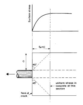
Fig 3. No-slip mechanism of cracking: relationship between C and  ${\rm S_0}$
