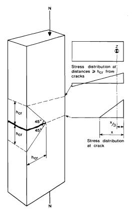
Fig 5. Cracking in an unreinforced member
