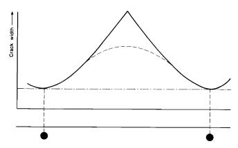
Fig 9. Variations in crack width in a member subjected to pure tension
