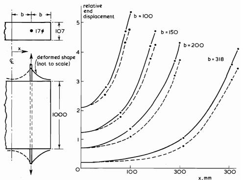
Fig 8. Finite element studies of crack width
