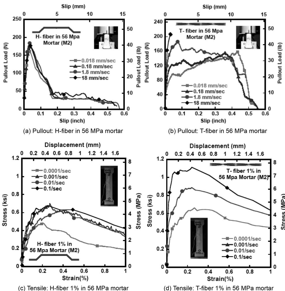
Fig. 7 Influence of fiber type on rate sensitive behavior of HPFRCC.<sup>29</sup>
