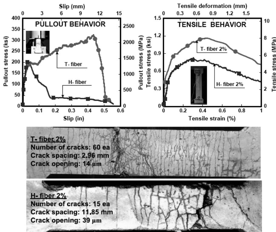
Fig. 3 Influence of different slip capacity on tensile properties of HPFRCC with 56 MPa mortar compressive strength.<sup>19</sup>
