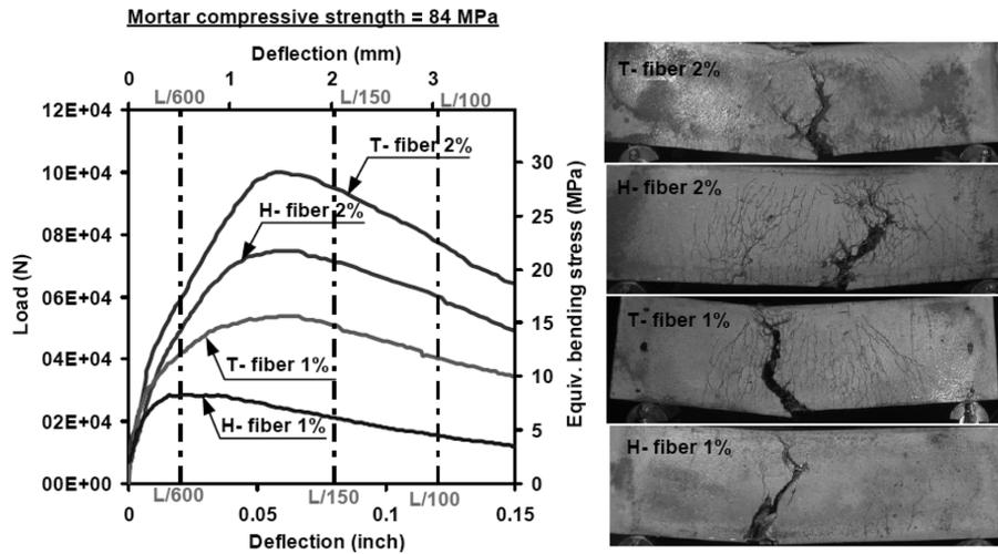
Fig. 4 Influence of different slip capacity on flexural behavior of HPFRCC with 84 MPa mortar compressive strength.<sup>22</sup>
