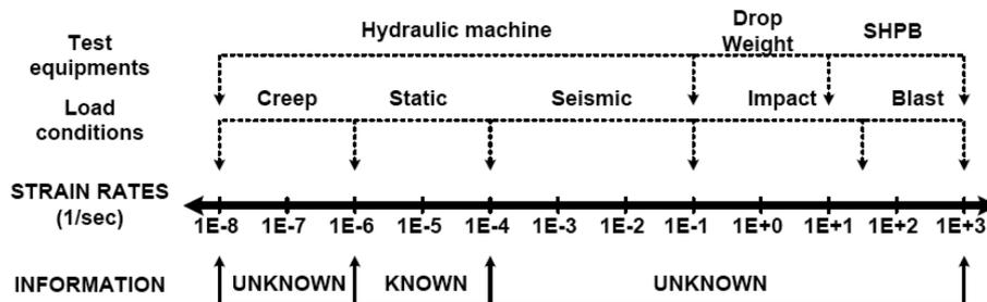
Fig. 6 Available test equipments and information for HPFRCC under various strain rates.
