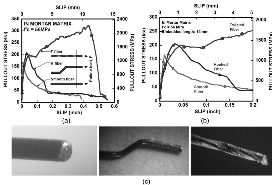
Fig. 2 Slip hardening and slip softening pullout behavior: (a) Entire pullout stress-slip curves; (b) Detail of initial portion of slip hardening and slip softening curves<sup>21</sup>; and (c) Photos for Smooth, Hooked and Twisted fibers.
