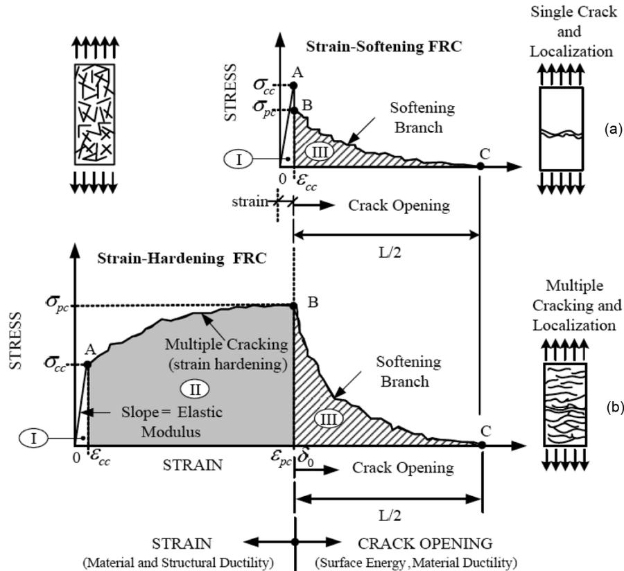
**Fig. 1** Typical stress-strain or elongation curve in tension up to complete separation: (a) Conventional strain-softening FRC composites; (b) Strain-hardening FRC composite or HPFRCC<sup>2,3,30</sup>
