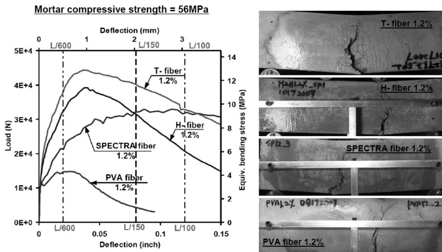
Fig. 5 Comparative flexural performance of four FRC composites.<sup>22</sup>
