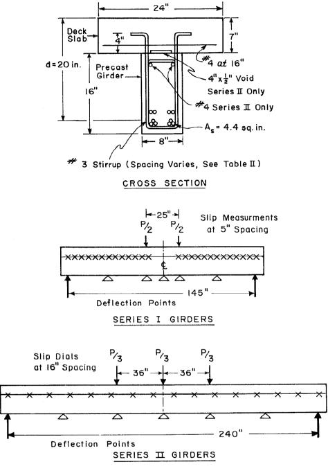
Fig. 9— Girder Test Specimens.
