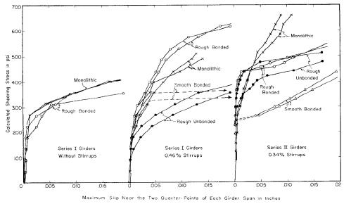
Fig. 17 — Shear-Slip Relationships for Test Girders.
