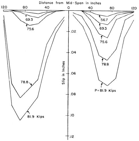
Fig. 16 — Typical Slip Development, Girder BRS-11.
