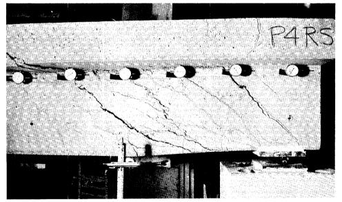
Fig. 14 — Diagonal Cracking in Series I.
