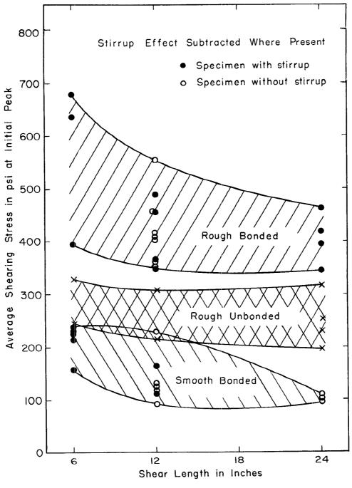
Fig. 7 --- Effect of Shear Length.
