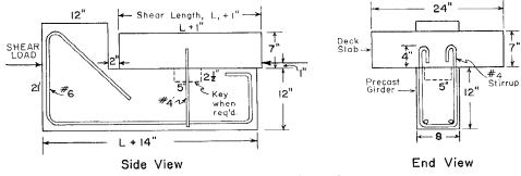
Fig. 1 — Pushoff Specimen in Casting Position.
