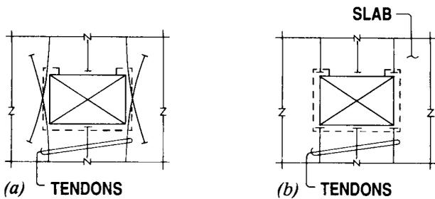
Fig. 5.1—Tendon layouts—(a) Crack inhibiting layout; and (b) crack promoting layout
