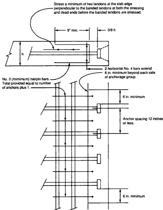
Fig. 3.5—Anchorage zone reinforcement for groups of  $\frac{1}{2}$  in. (13 mm)  $\phi$  270 k (1862 MPa) monostrand tendon anchorages in slabs<sup>40</sup>
