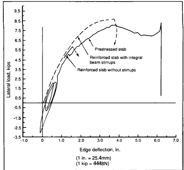
Fig. 2.1—Comparison of lateral load-edge deflection relationships for reinforced and prestressed concrete slab-interior column specimen<sup>11</sup>
