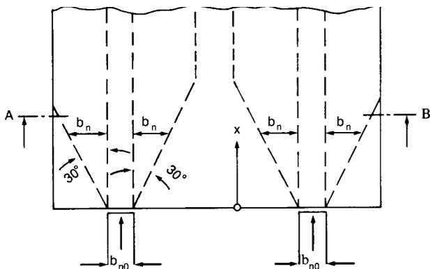
Fig. 3.2—Effective flange widths for normal forces
