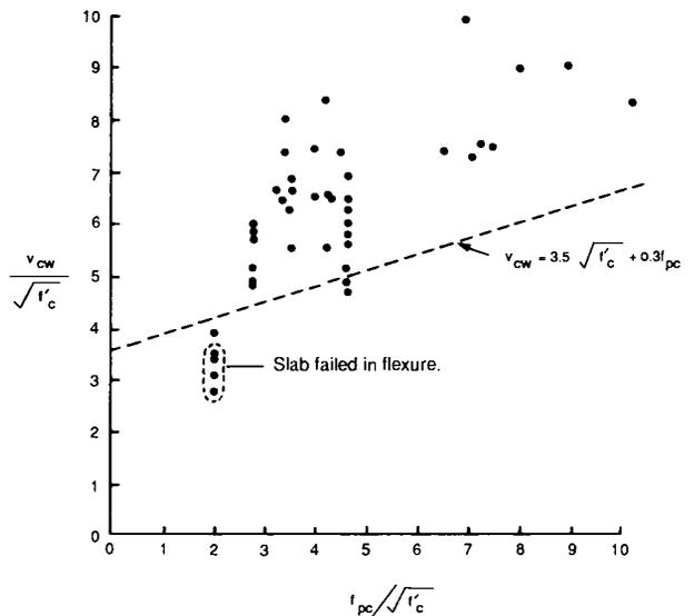
Fig. 3.3—Two-way flat plate shear test data versus Eq. (11-37) of ACI 318<sup>27</sup>
