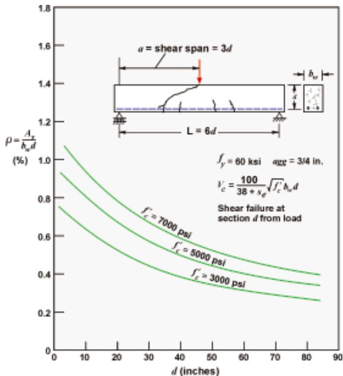
Fig. 14: Percentage of longitudinal reinforcement above which a beam without stirrups will fail in shear (1 in. = 25.4 mm; 1 ksi = 6.89 MPa; and 1 psi = 6.89 kPa)
