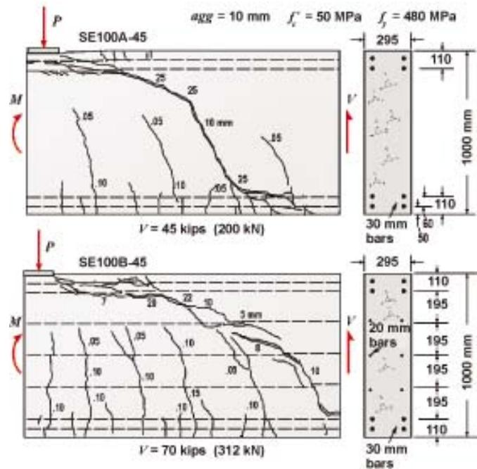
Fig. 7: Influence of distribution of longitudinal reinforcement on cracking pattern and shear strength of two companion beams
