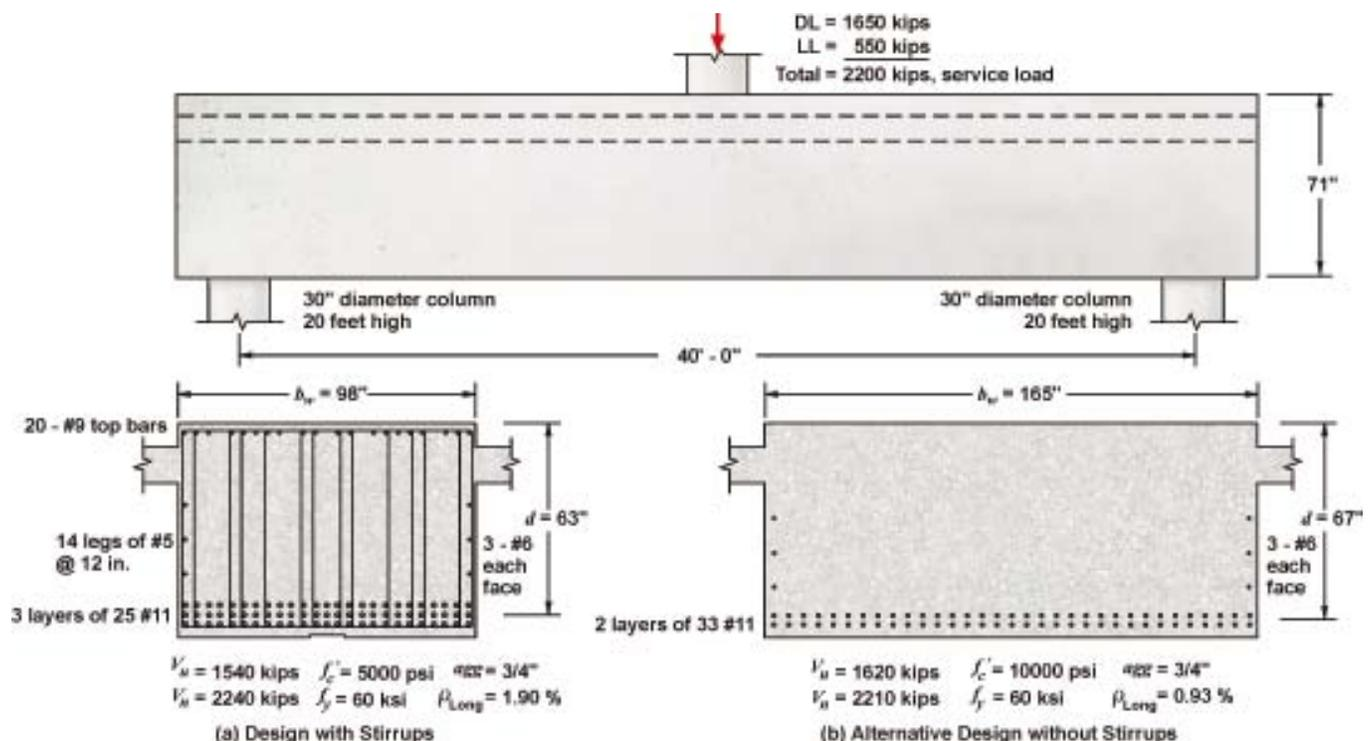
Fig. 1: Shear design of transfer beams at the Bahen Center (1 in. = 25.4 mm; 1 ksi = 6.89 MPa; 1 psi = 6.89 kPa; 1 k = 4.45 kN)
