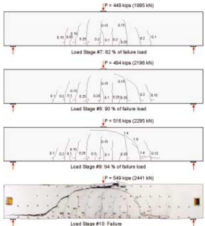
Fig. 11: Crack development with crack widths in millimeters for Beam AT-1
