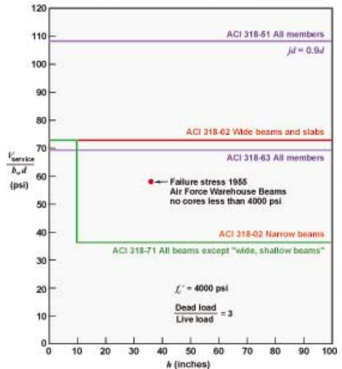
Fig. 4: Service load stress at which stirrups are not required (1 in. = 25.4 mm; 1 psi = 6.89 kPa)
