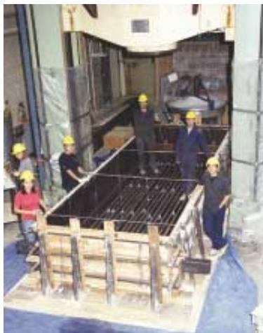
Fig. 8: Construction and loading of the large, wide beam, AT-1 under testing machine at the University of Toronto
