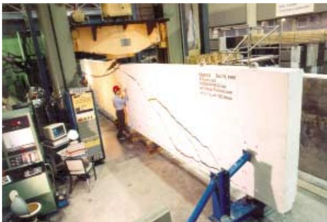
Fig. 16: Failure of large beam at 47% of ACI shear failure load
