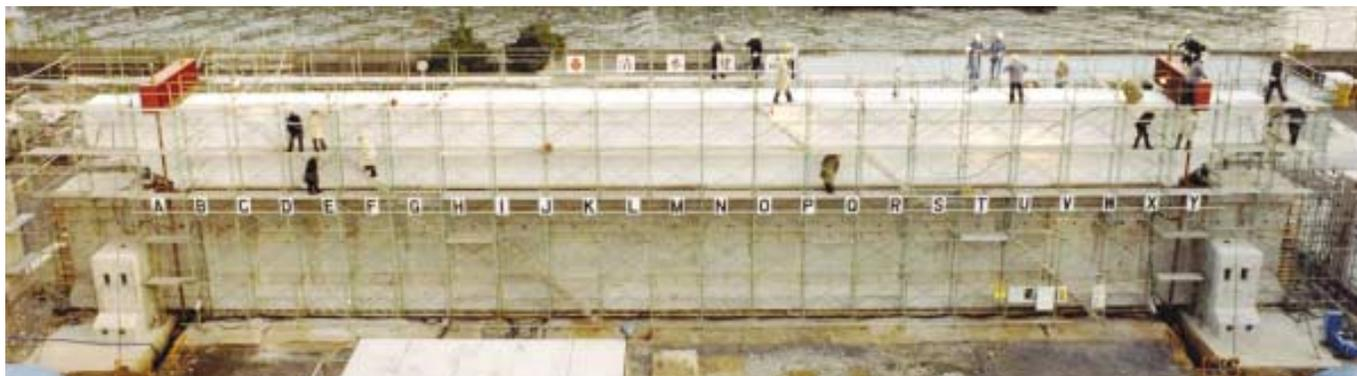
Fig. 6: Large beam failing in shear. Failure crack between S and X (photo courtesy of Shimizu Corp.)
