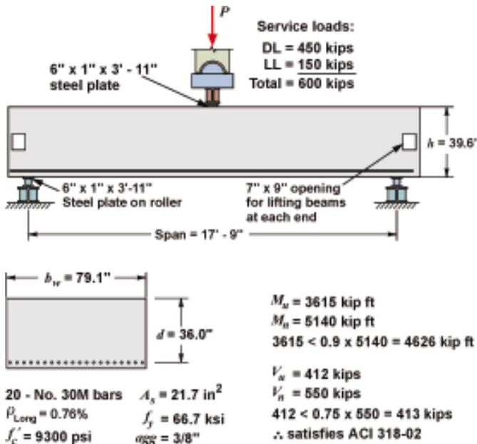
Fig. 9: Design of test Beam AT-1 (1 in. = 25.4 mm; 1 ksi = 6.89 MPa; 1 psi = 6.89 kPa; 1 in<sup>2</sup> = 645 mm<sup>2</sup>; 1 k = 4.45 kN; and 1 ft-k = 1.354 kNm)
