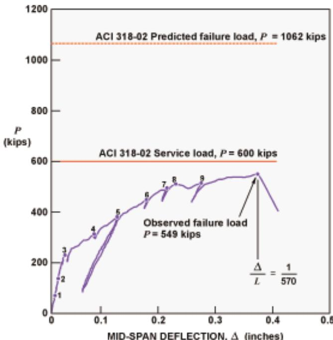
Fig. 10: Observed load-deformation response of Beam AT-1 (1 in. = 25.4 mm; 1 k = 4.45 kN)
