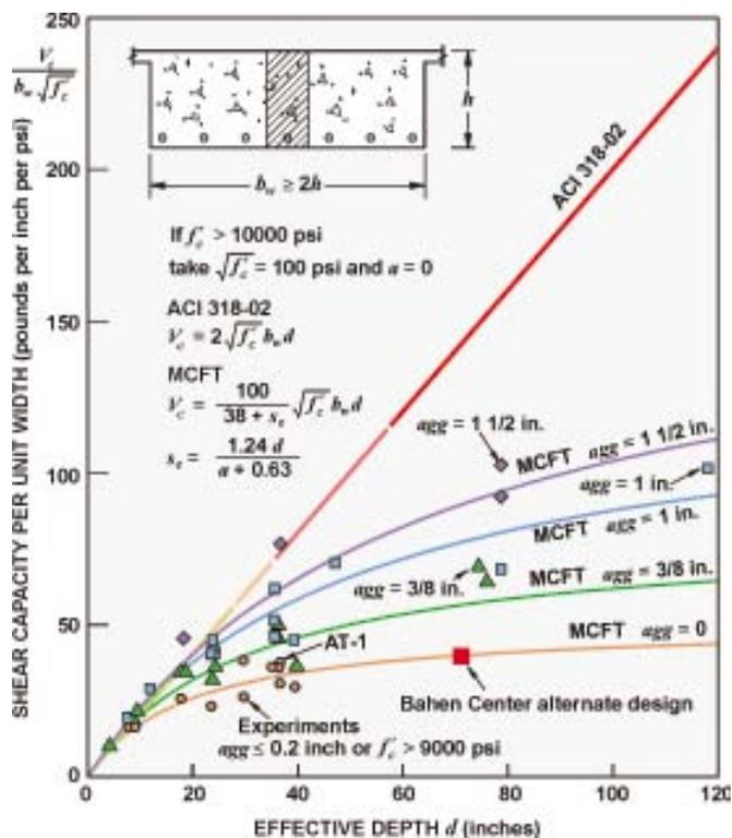
Fig. 13: Safety of ACI shear design procedure for large, wide beams (1 in. = 25.4 mm; 1 lb/in.<sup>2</sup> = 0.025 kN/m<sup>2</sup>/kPa; and 1 psi = 6.89 kPa)
