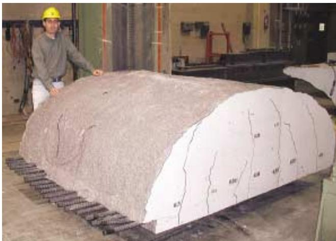
Fig. 12: Failure surface of Beam AT-1. Note, reinforcing bars have been cut
