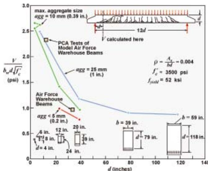
Fig. 5: Influence of member depth and maximum aggregate size on shear stress at failure (tests by Shioya et al.<sup>9</sup> and Shioya<sup>10</sup>) (1 in. = 25.4 mm; 1 ksi = 6.89 MPa; 1 psi = 6.89 kPa)
