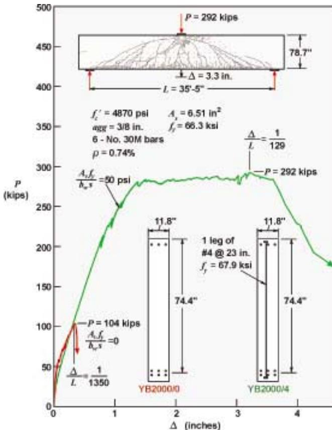
Fig. 15: Influence of minimum shear reinforcement on load-deformation response of large beams (1 in. = 25.4 mm; 1 ksi = 6.89 MPa; 1 psi = 6.89 kPa; 1 in.<sup>2</sup> = 645 mm<sup>2</sup>; and 1 k = 4.45 kN)
