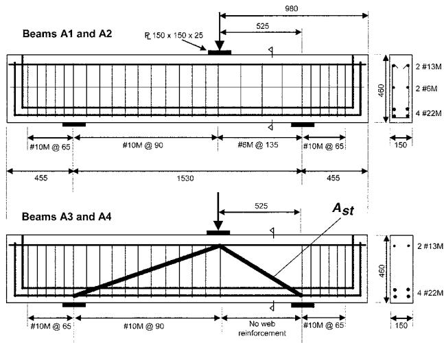
Fig. B—Reinforcement details for Series A.
