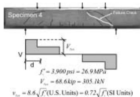
Fig. 7—Failure conditions of Specimen 4.
