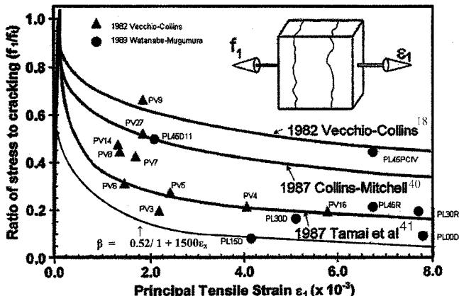
Fig. A—Ratio or stress to cracking ( $f_1/f_v$ ) versus principal tensile strain  $\epsilon_1$  ( $\times 10^{-3}$ ).<sup>39</sup>
