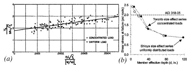
Fig. D—Comparison of shear strengths of uniformly loaded and point loaded members for: (a) small heavily reinforced members; and (b) large lightly reinforced members.
