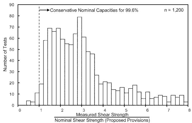
Fig. 21—Distribution of shear strengths calculated using proposed provisions for full database.
