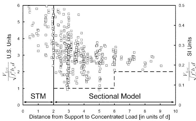
Fig. 18—Proposed shear strength provisions for sectional models for members subjected to concentrated loads.
