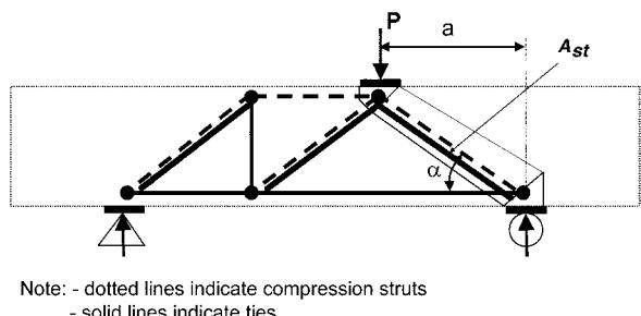
Fig. A—Strut-and-tie model for deep beam design.
