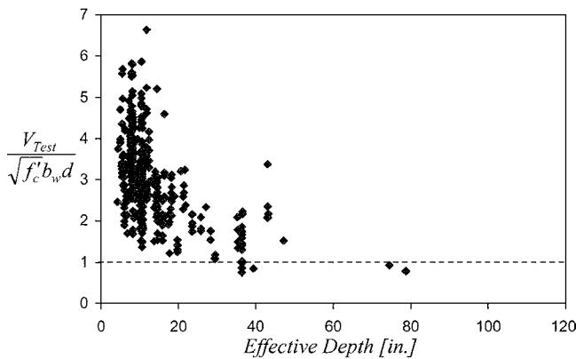
Fig. F—Shear strength versus effective depth based on Reineck et al.<sup>62</sup> database.
