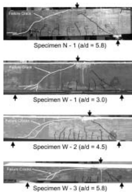
Fig. 13—Photographs of asymmetric tests after failure (for all specimen  $a/d = 1.7$  for right side;  $a/d$  ratios listed within figure refer to left side).
