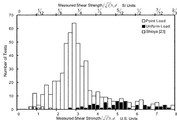
Fig. 14—Shear strength of specimens without web reinforcement.
