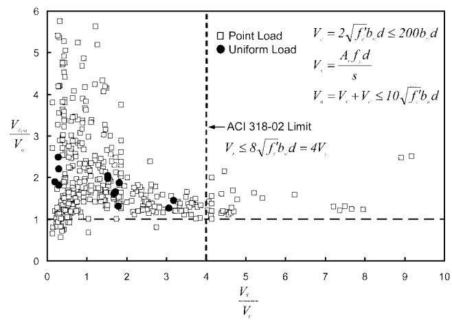
Fig. 19—Effect of transverse reinforcement for all specimens with  $V_s > 0$ .
