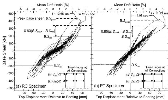
\*  $B.S_{res}$ , Residual base shear of the frame calculated assuming that all the connections are perfectly hinged
