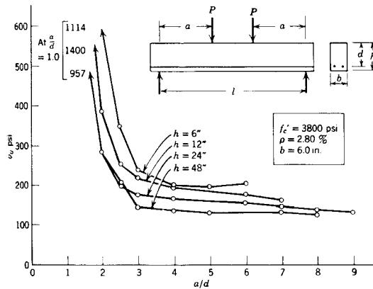
Fig. 3—Relationship between shear span-to-depth ratio and shear strength.<sup>5</sup>
