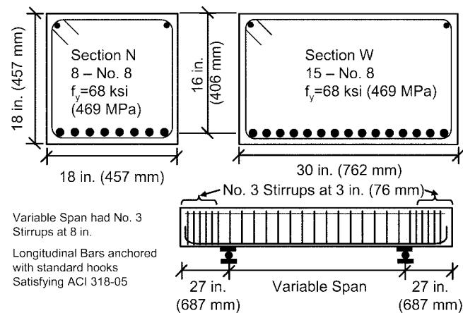
Fig. 12—Details of asymmetric concentrated load tests.
