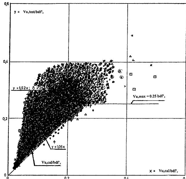
Fig. B—Test shear failure  $V_{u,test}$  compared with calculated shear capacity  $V_{u,cal}$ .<sup>54</sup>
