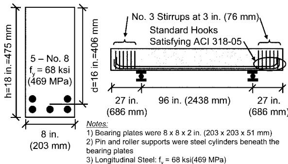
Fig. 4—Details of test Specimens 1, 2, 4, and U.
