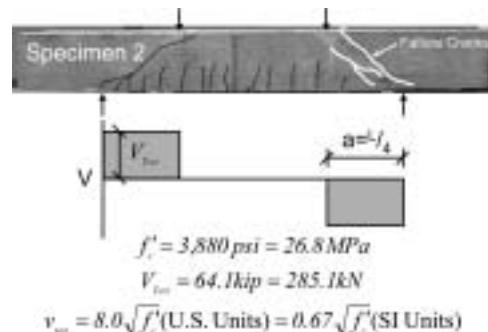
Fig. 6—Failure conditions of Specimen 2.
