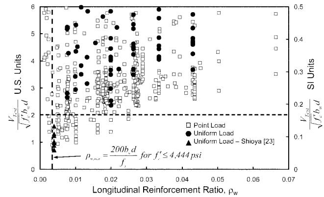
Fig. 15—Concrete contribution to shear strength versus longitudinal reinforcement ratio.
