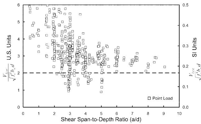
Fig. 17—Shear strength of specimens without web reinforcement.
