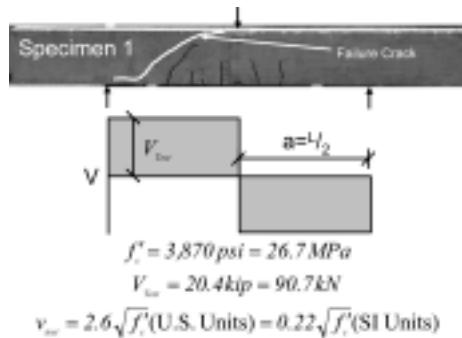
Fig. 5—Failure conditions of Specimen 1.
