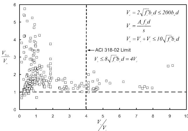
Fig. 20—Effect of transverse reinforcement for specimens with point loads that satisfy ACI 318-05 spacing requirements and minimum shear reinforcement requirements.
