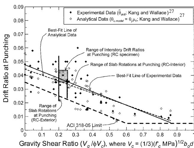
Fig. C—Drift ratio at punching versus gravity shear ratio (reinforced concrete interior connections without shear reinforcement and reinforced concrete shaketable specimen).
