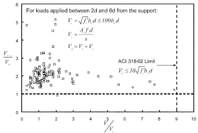
Fig. 22—Maximum shear strength using proposed shear provisions for specimens that satisfy ACI 318-05 spacing requirements and minimum shear reinforcement requirements and subjected to concentrated loads.
