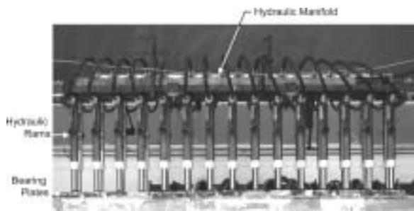
Fig. 10—Hydraulic rams used for uniform load.
