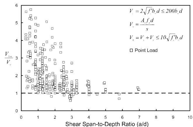
Fig. 16—Shear strength of specimens with web reinforcement.
