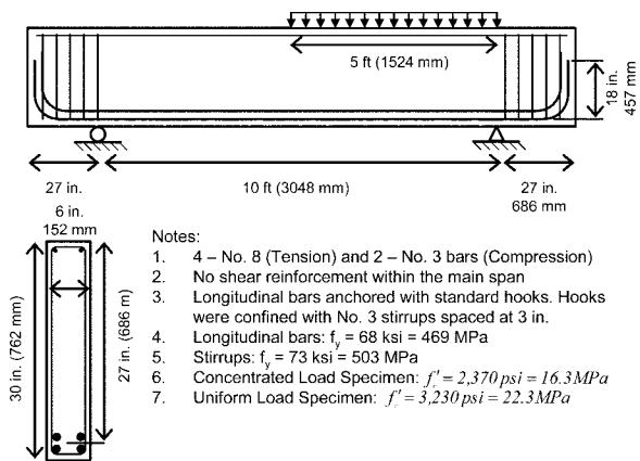
Fig. 9—Specimens used to examine strain distribution.
