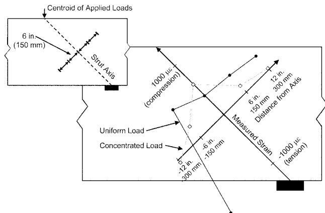
Fig. 11—Location of strain gauges (inset top left) and measured strain values.
