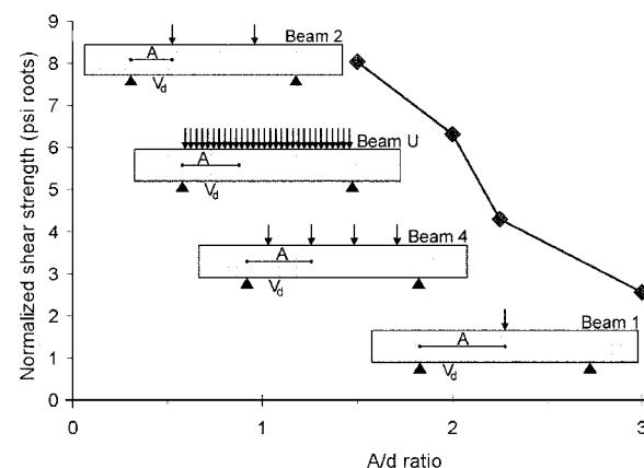
Fig. C—Shear strength of authors' tests with respect to shear span.
