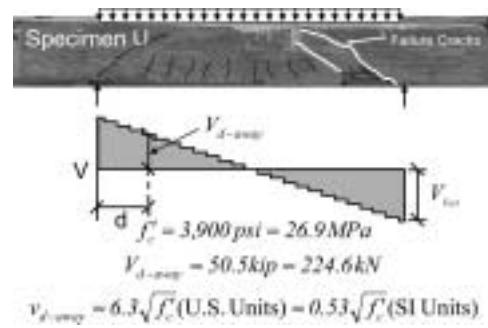
Fig. 8—Failure conditions of Specimen U.
