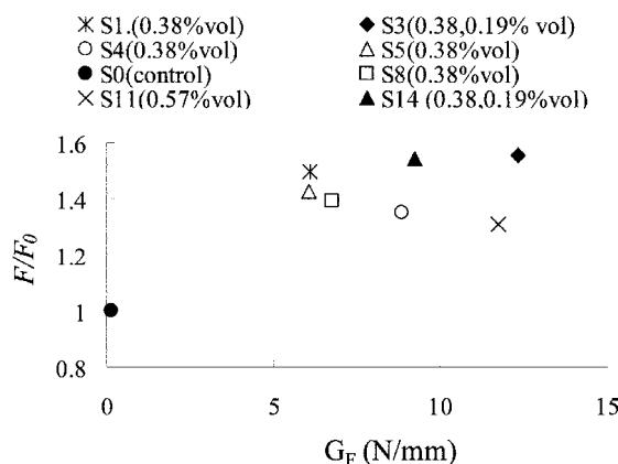
Fig. A— $F/F_0$  varies with fracture energy  $G_F$ .
