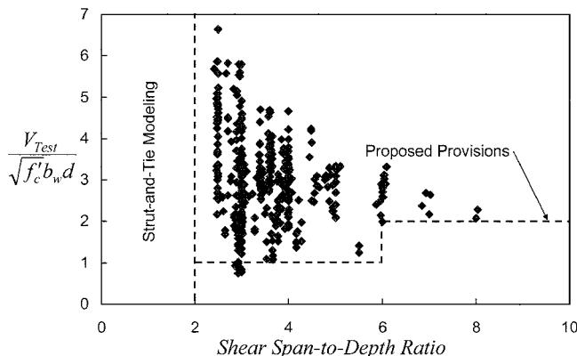
Fig. G—Shear strength versus shear span-to-depth ratio based on Reineck et al.<sup>62</sup> database.
