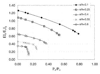
Fig. 6—Influence of eccentricity ratio and axial load ratio on effective I of columns ( $\rho_g = 1\%$  and  $f_c' = 4000$  psi).
