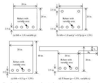
*Fig.* 8—*Cross section of typical reinforced concrete beams considered in parametric study.*
