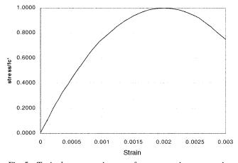
Fig. 5—Typical stress-strain curve for concrete in compression.
