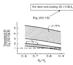
Fig. 11—Comparison of ACI 318-95, Eq. (10-13) (same as Eq. (10-12) in ACI 318-02) for EI with EI values from momentcurvature diagrams (MacGregor, Breen, and Pfrang 1970).
