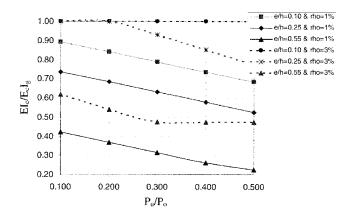
Fig. 12—Influence of axial load and eccentricity ratio on flexural stiffness of columns.
