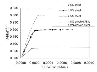
Fig. 9—Moment-curvature relationships for typical reinforced concrete beams: influence of tensile reinforcement ratio.
