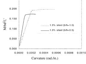
*Fig.* 10—Moment-curvature relationship for typical reinforced concrete beams: influence of aspect ratio b/h.
