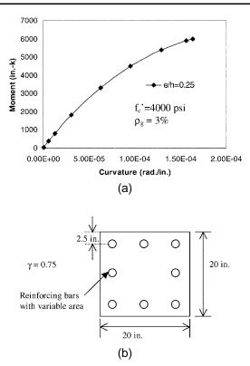
Fig. 2—(a) Moment-curvature relationship for typical reinforced concrete column considered in parametric study (for e/h ratio of 0.25 and reinforcement ratio of 3%); and (b) cross section of typical reinforced concrete column considered in parametric study.
