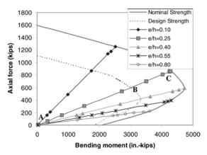
Fig. 4—P-M interaction diagram and loading histories for typical column ( $\rho_g = 1\%$  and  $f_c' = 4000$  psi).
