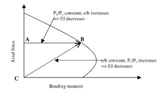
Fig. 7—Influence of axial load and eccentricity ratios on moment of inertia of columns.
