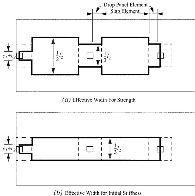
Fig. 2—Effective slab widths for strength and stiffness.
