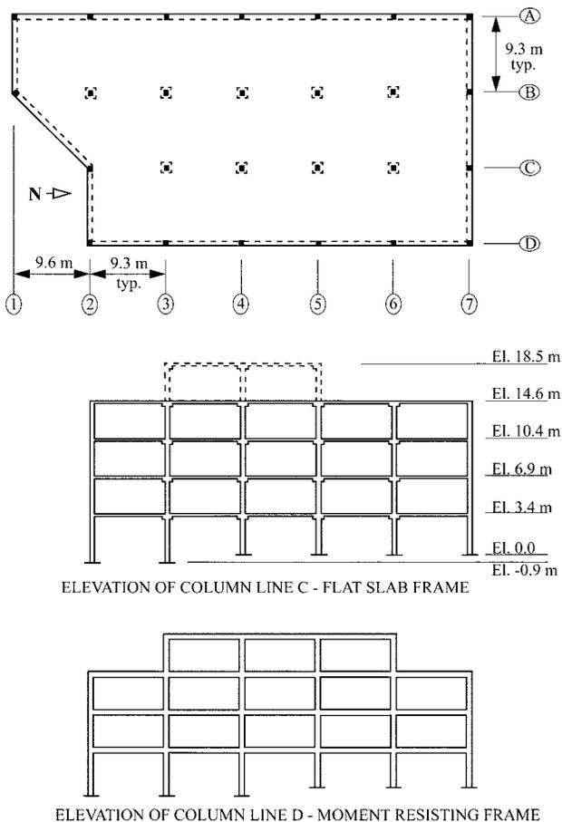
Fig. 4—Office building first-floor plan and two superstructure frame elevations.
