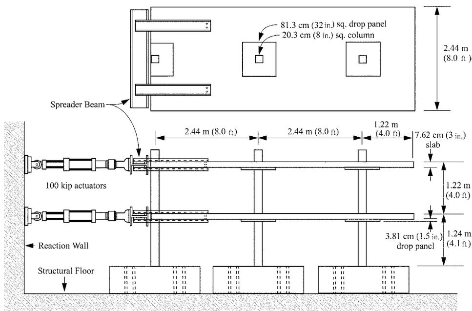
Fig. 1—Two-story, two-bay frame test setup.
