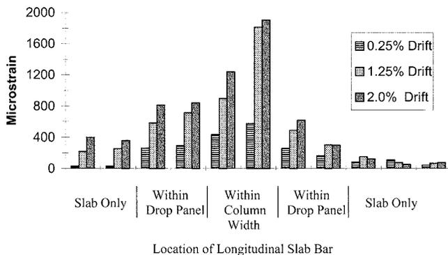
Fig. 3—Measured strain range per cycle in top longitudinal bars across transverse width of slab.
