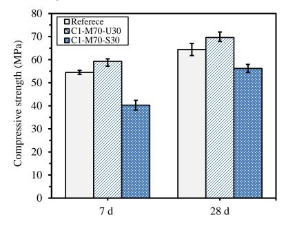
✓ ~ 16% and 11% higher compressive strength in concrete with 50 wt% MK-UFS compared to that concrete with only cement at 7 and 28 d, respectively
