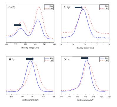
Decrease in the values of binding energy of elements after ultrafine grinding
