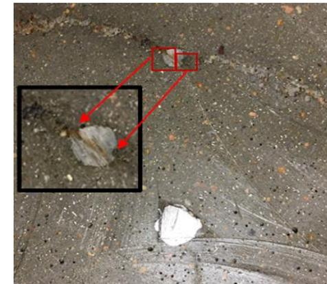
Corrosion of steel reinforcement (crack width > 0.1 mm)
