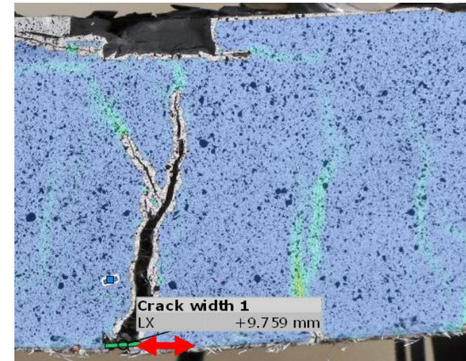
Defining two points on either side of widest crack at maximum load
