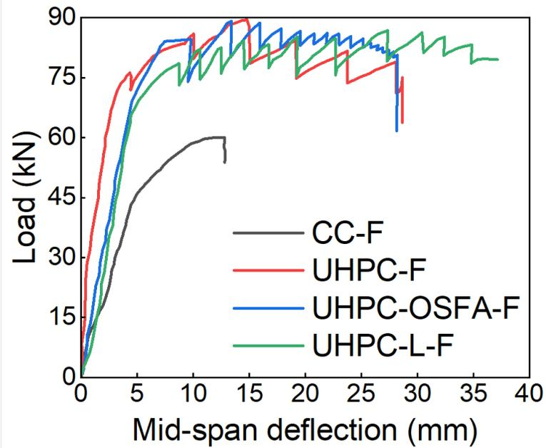
Beams without shear reinforcement
