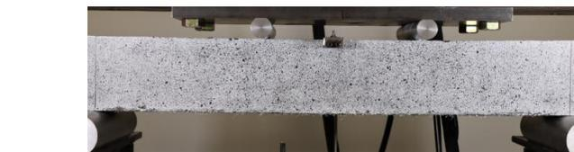
UHPC-OSFA-F beam Load: 21 kN
