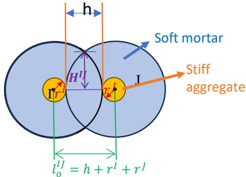
$$l^{IJ} = l_o^{IJ} \quad P=h \text{ then } F_n=0 \text{ ( zero configuration)}$$
