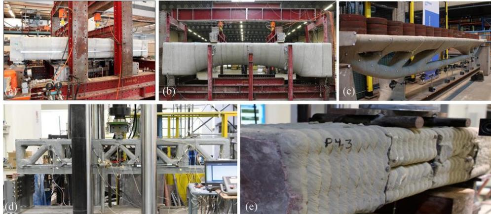
Fig. 14. 3DPC spliced beams in different experimental states: (a) Scale model specimen in bending set-up (Salet et al., 2018), (b) Setup of the structural mock-up test (Ahmed et al., 2022), (c) Uniform load test on post-tensioned prestressed girder (Vantighem et al., 2020), (d) Straight beam for the three-point bending test (Asprone et al., 2018), (e) Failure pattern for 3DPC beam (Assaad et al., 2020).
