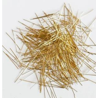
Steel Fibers \phi = 200 \mu\text{m} , L = 13 \text{ mm}
