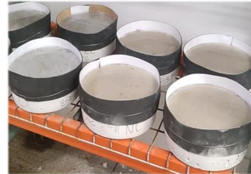
Diked specimen ponded with chloride solution
