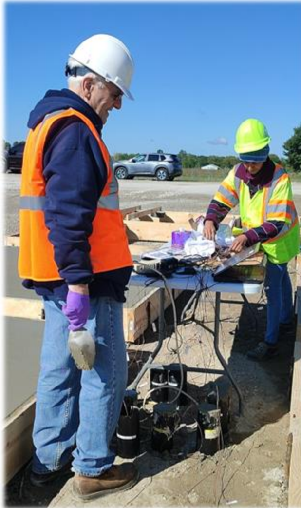
cylinders connected to Data logger
