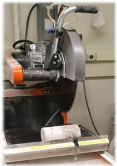
Cutting cores to dimension
