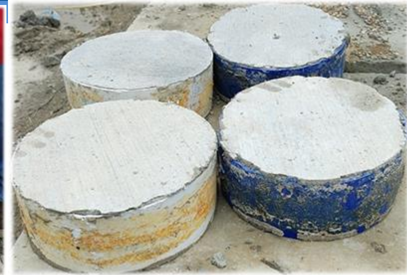
Specimen for scaling resistance test
