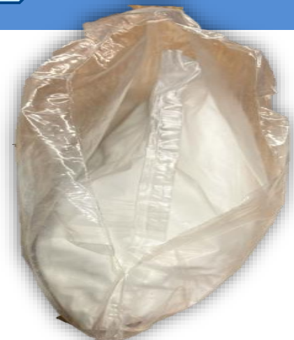
Superabsorbent polymer Polyacrylamide-based particles Dry diameter < 300 \mu\text{m}
