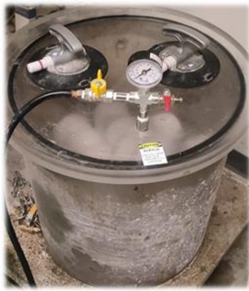
Vacuum-saturation of cores
