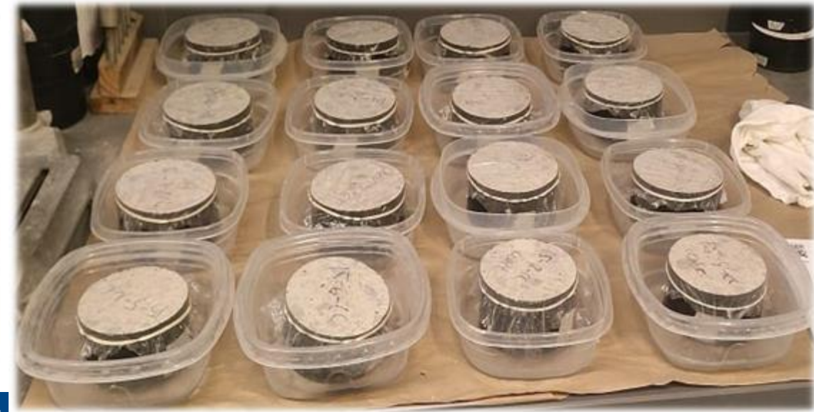
Evaluation of the rate of water absorption of test specimens
