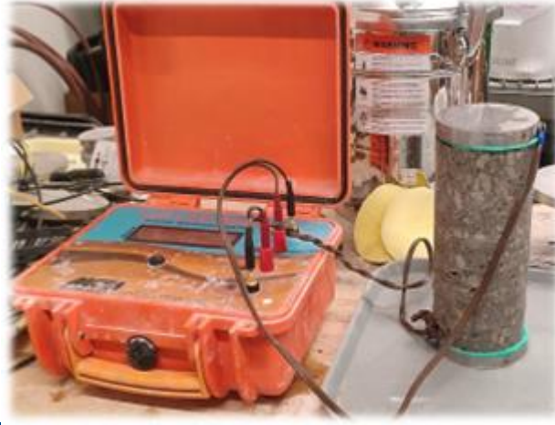
Electrical Resistivity Testing
