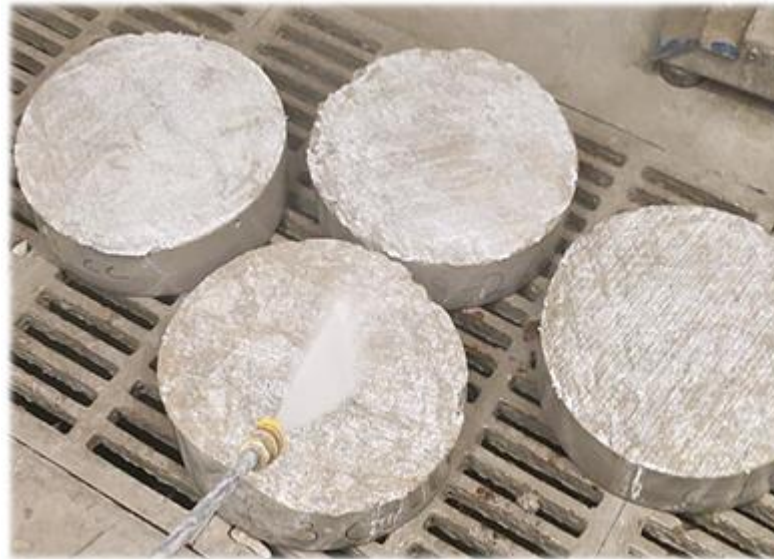
Power washing of test specimen
