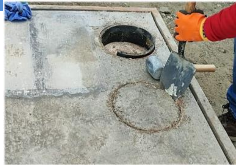
Extraction of test specimen from the field
