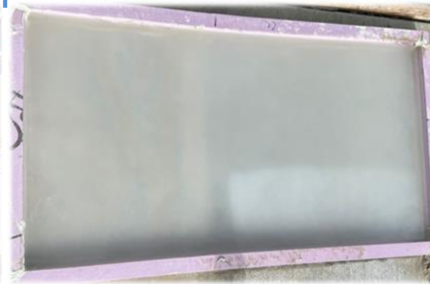
Field-cast slab ponded with chloride solution
