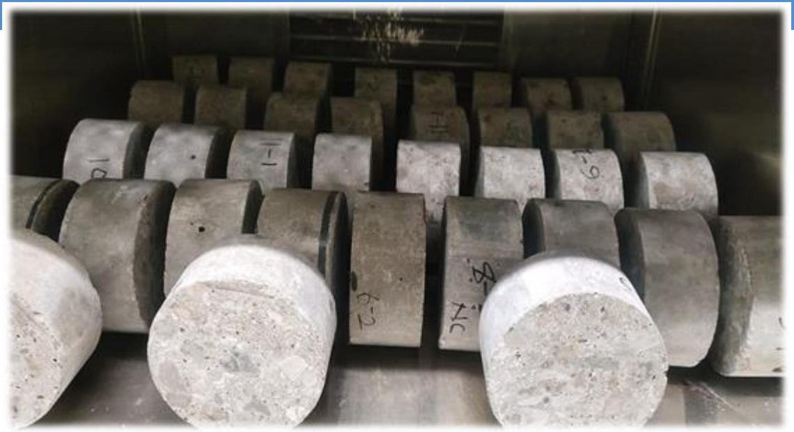
Cores drying in the environmental chamber
