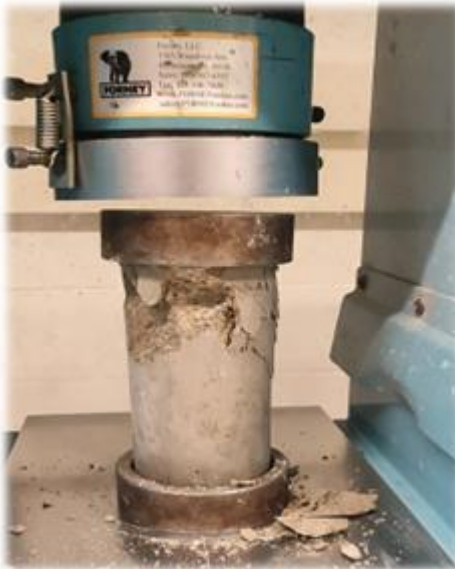
Compressive Strength Testing
