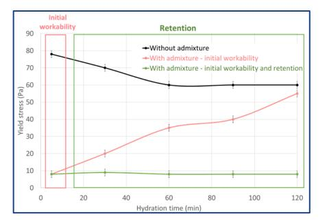
**65 wt% cement + 35 wt% calcined clay // W/B = 0.39** Rheometer measurement of shear stress for shear rate from 200 to 0.01 s-1 // Yield stress determination at the minimum shear stress
