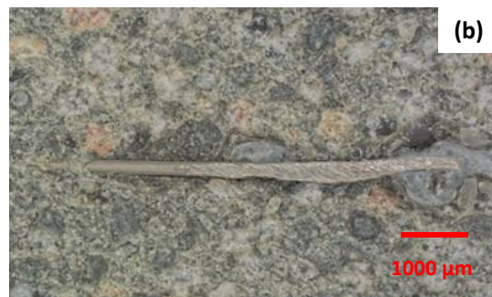
Representative section parallel to: (a) X-Z plane, and (b) X-Y plane for printed UB-SF 1.5%
