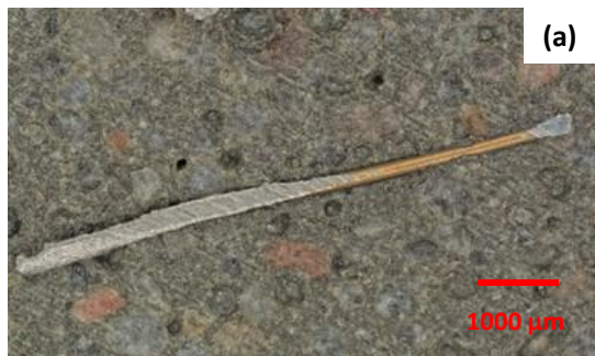
Representative section parallel to: (a) X-Z plane, and (b) X-Y plane for printed UB-SF 1.5%
