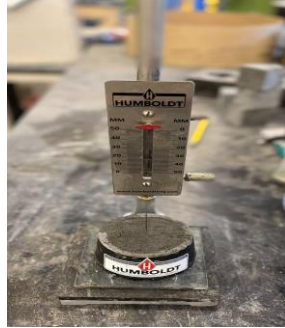
Setting Time (ASTM C191-21)
