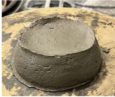
Flow Table Test (ASTM C230/C230 M-21)
