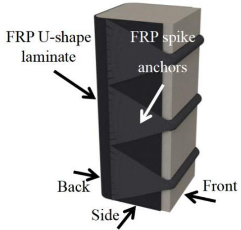
Stage 1: testing on prism
