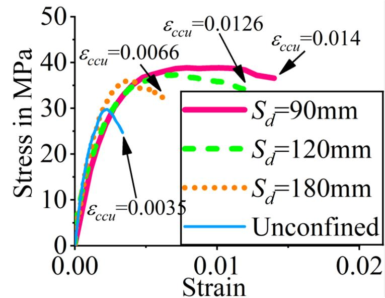
**Key finding:** the confined concrete exhibited an improved strength capacity by 1/3 and strain capacity by 4 times, when the anchor spacing was 90 mm.
