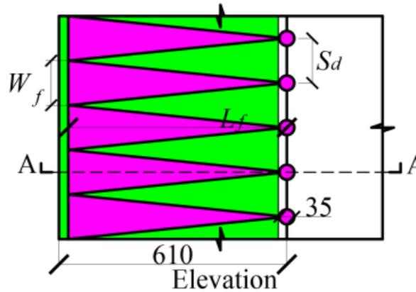
$$N_{fr} = 3.6 \times 236.4 \times 10^3 \text{ MPa} \times 0.00118 \times (254.5)^{0.56} \text{ mm}^2 \times \frac{90^\circ - \frac{180^\circ}{\pi} \arctan\left(\frac{0.5 \times 120}{610 - 25}\right)}{90^\circ} = 208.8 \text{ kN}$$
