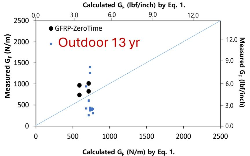
Same observation: several factors affect measured  $G_F$  -- concrete strength, environment, sustained loading, and **position where  $G_F$  measured**
