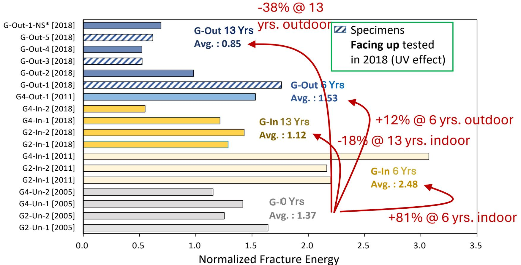
\*G-Out-1-NS [2018] is a GFRP specimen that was outdoors for 13 years without sustained load
