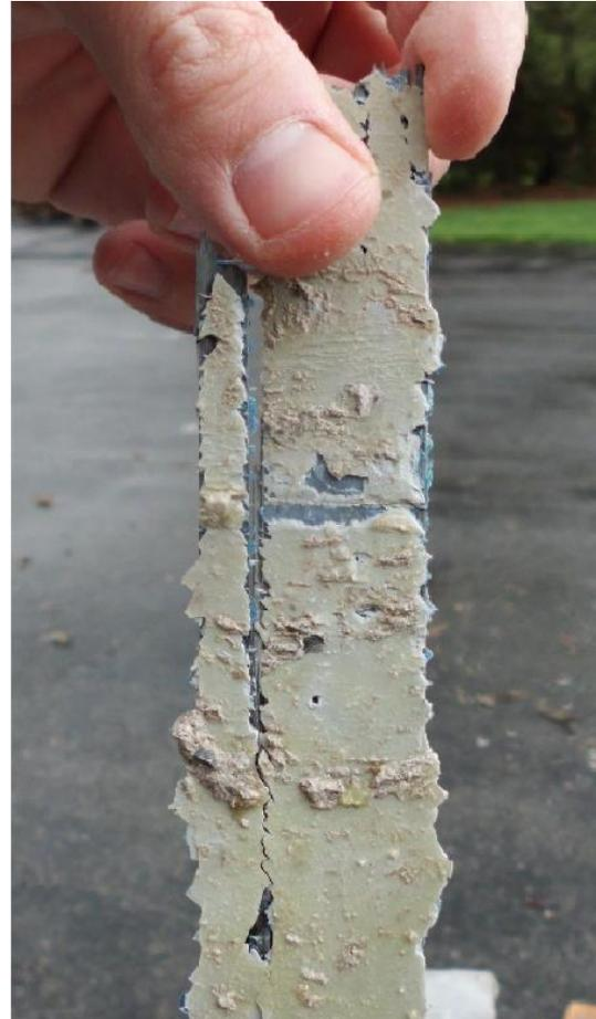
Mix of adhesive failure and concrete-cohesive failure
