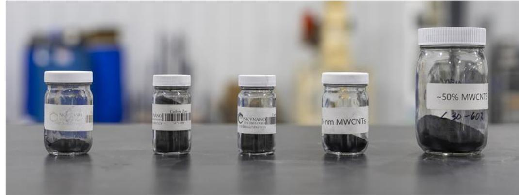
The SkyNano technology of MWCNT production is based on molten salt electrolysis, where carbonate-ion reduction occurs at the cathode and oxide-ion oxidation occurs at the anode. The captured CO<sub>2</sub> is then used to chemically regenerate the molten salt electrolyte by converting excess oxide ions back to carbonate ions.
