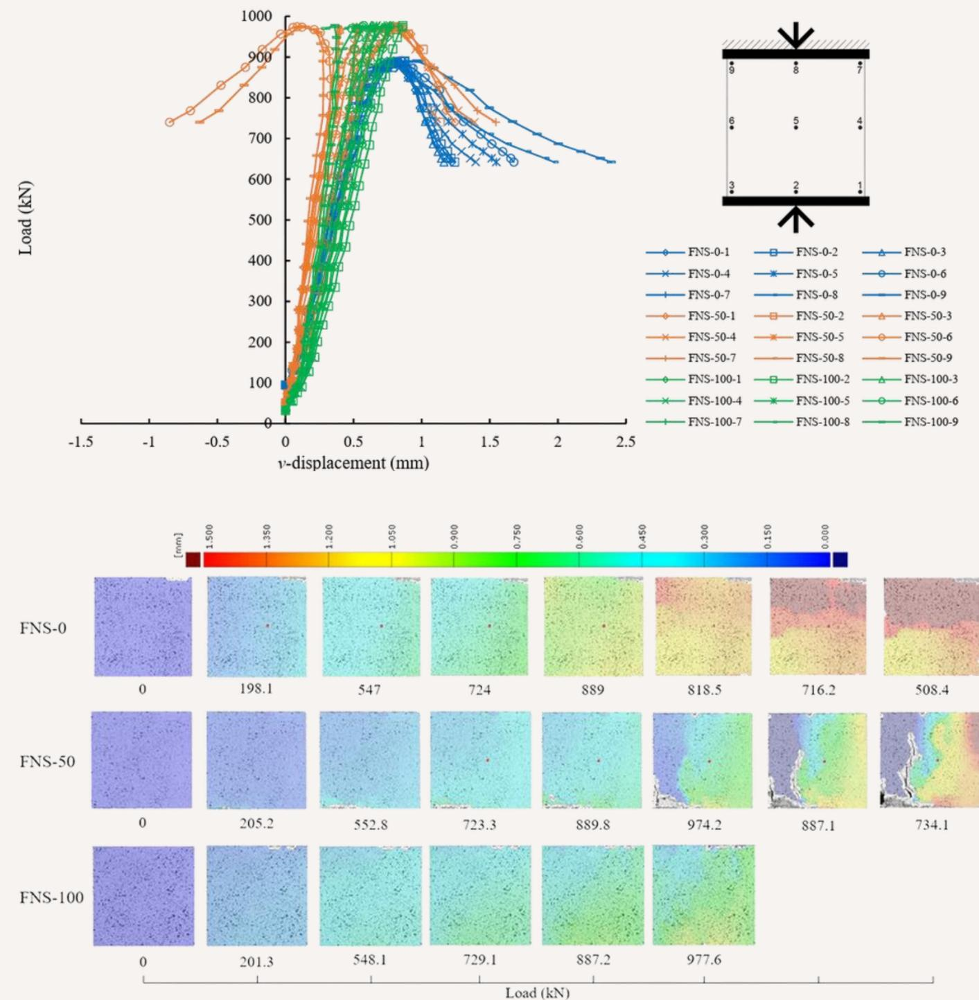
Figure 10. v-displacement field of cubic specimens.
