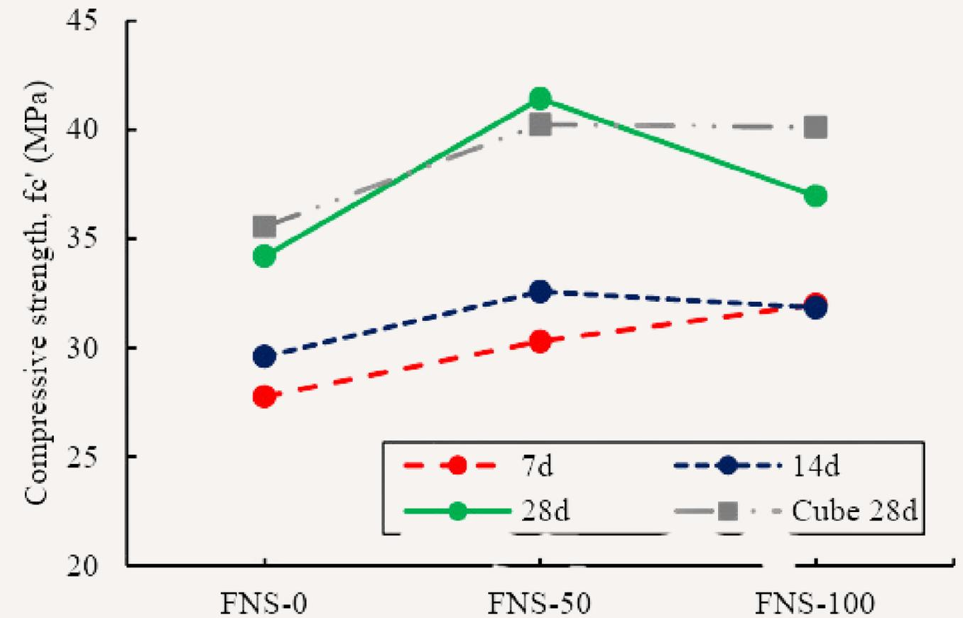
Figure 6. Effects of FNS substitution on compressive strength.
