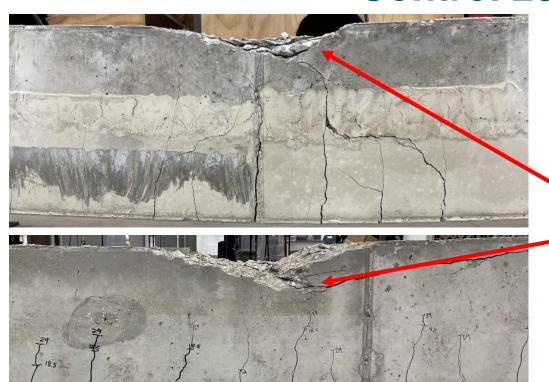
Flexural failure ending with concrete crushing
