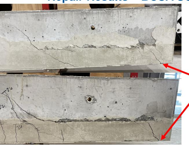
Diagonal tension cracks start at support locations
