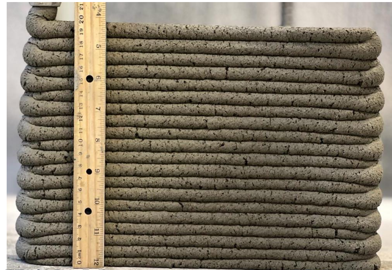
Height Measurement after 23 layers
