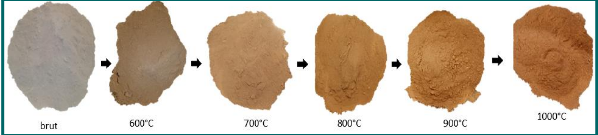
Change in color of the sediments at various temperature
