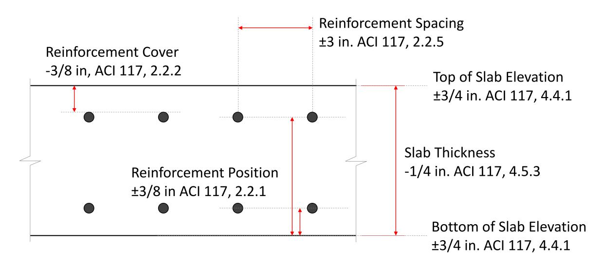
ACI 117-10(2015) "Specification for Tolerances for Concrete Construction and Materials"
