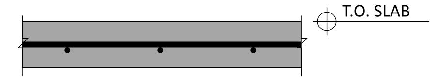
Thickness of suspended slab (ACI 117-10, Section 4.5.3): -1/4 in., no plus tolerance
