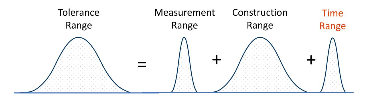
• Structures move, so when tolerances are measured for evaluation can be critical
