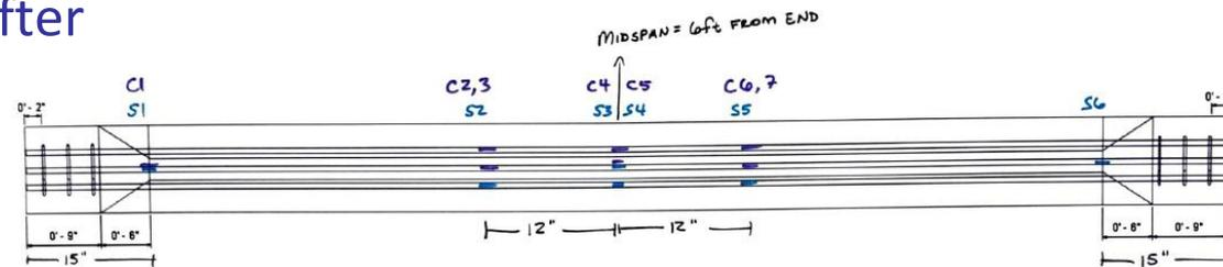
Sample pile instrumentation
