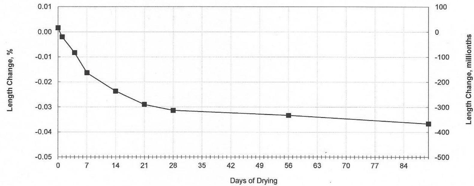
ASTM C1107/C1107M-20 specifies that a Nonshrink Hydraulic Cement Grout shall not have a change in length of more than 0.3% at 28 days.
