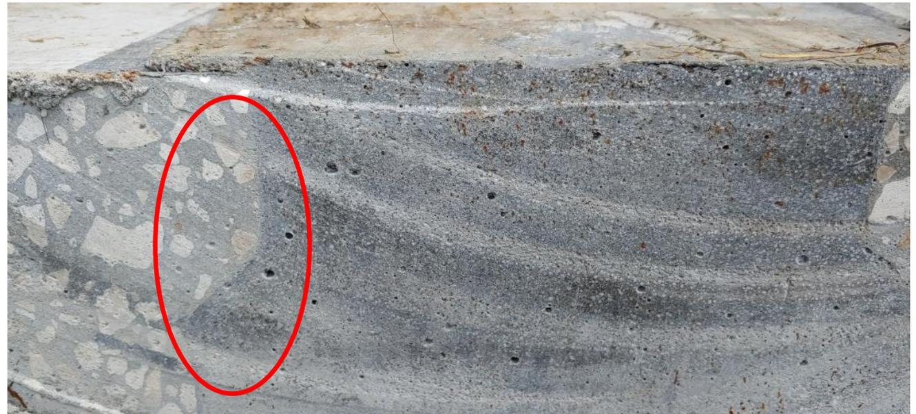
UHPC Interface Bond to Normal Concrete.
