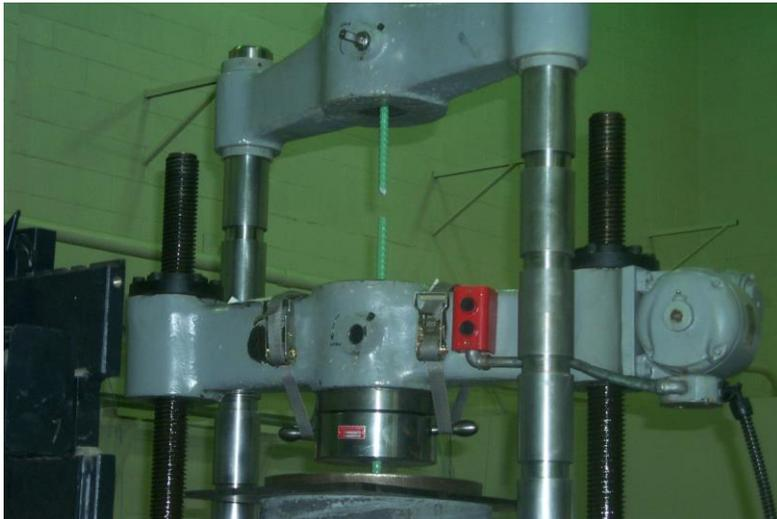
Bar Rupture with  $4 d_b$  in UHPC @ 14,000 psi.
