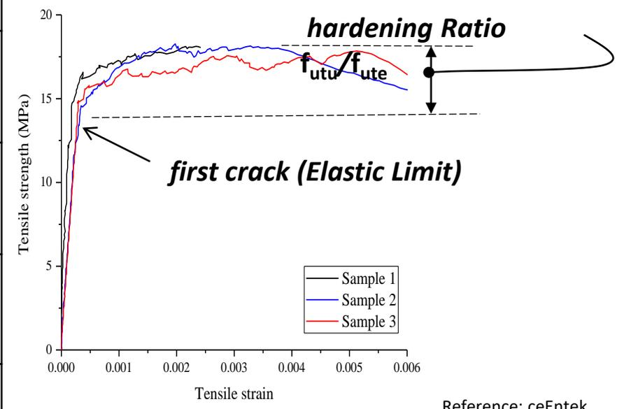
**Ultra-high performance concrete (UHPC)** — a cementitious composite material with enhanced strength, durability, and ductility compared to high performance concretes.
