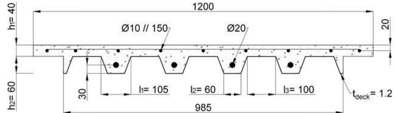
***Suspension bridge decks are designed to be light in weight to reduce deadload on the suspension cables and stiff to resist movement (bending & torsion) from wind and traffic. This results in very thin composite decks, with a potential for punch through if too much of the existing concrete material is removed during rehabilitation.***
