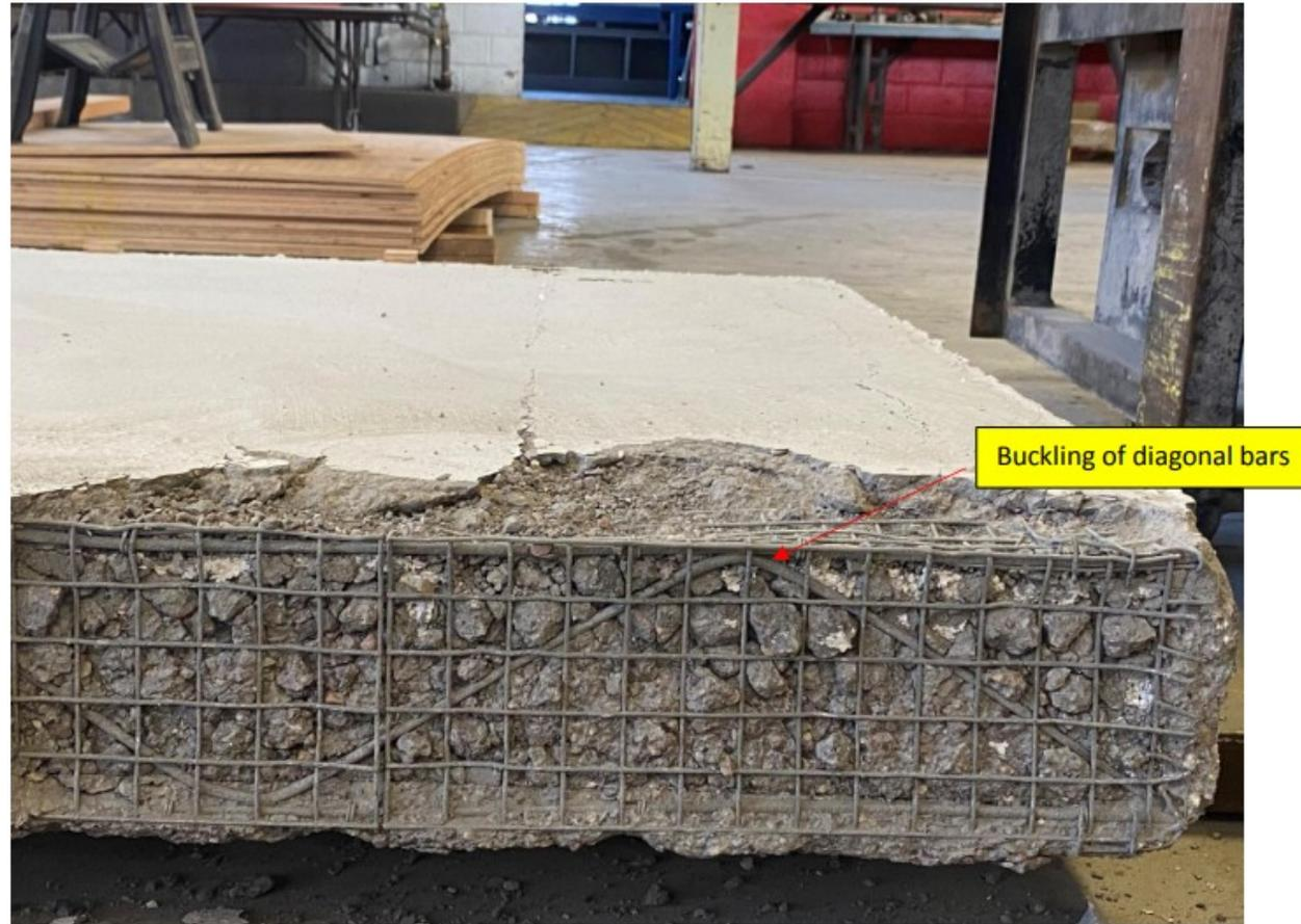
Figure 16. Buckling of panel 2
