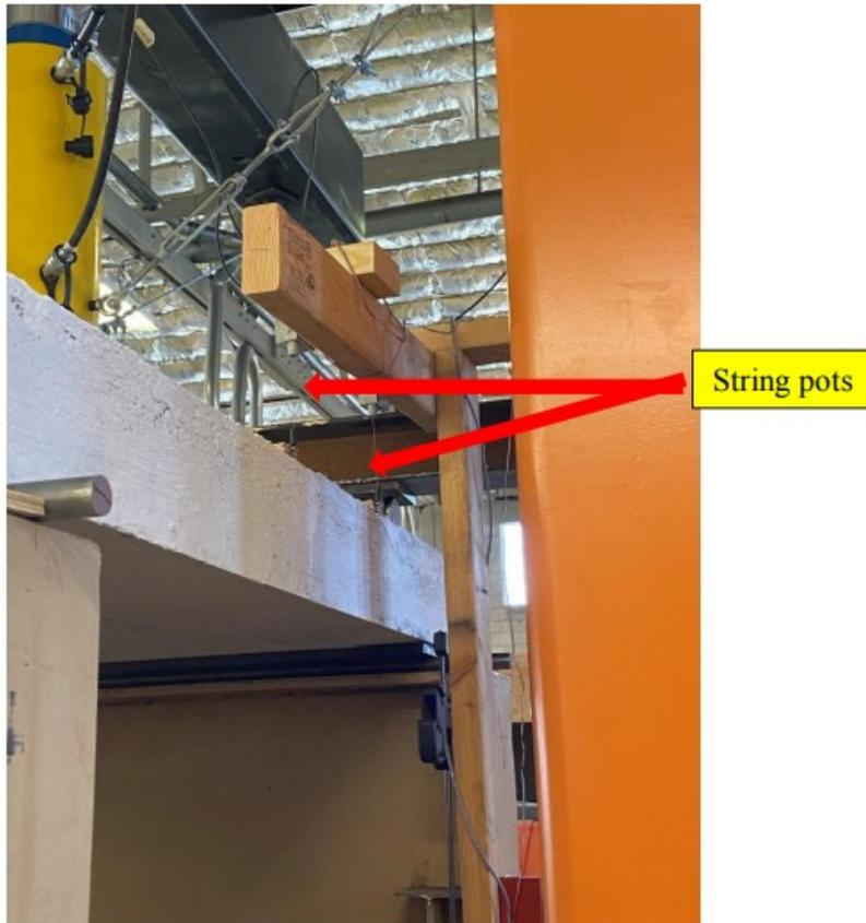
Figure 10. String pots attached on the specimen
