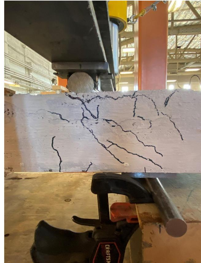
Figure 15. Shear cracks on before and after test on east edge of panel 2
