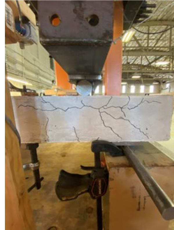
**Figure 13.** Shear cracks on before and after test on east edge panel 1
