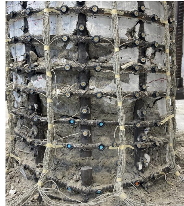
Smooth Bar in the Plastic Hinge
