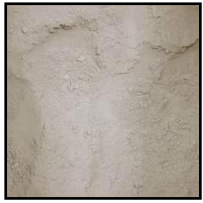
Binder (Cement, Fly Ash, Silica Fume, Glass Quartz)
