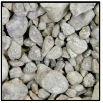
Coarse Aggregate (Crushed Stone)
