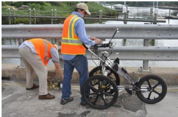
Radar testing of bridge deck.
