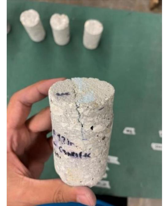
Fig. 11. Concrete core
