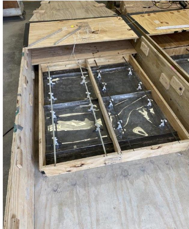
*Fig. 7. Mold and reinforcement configuration*
