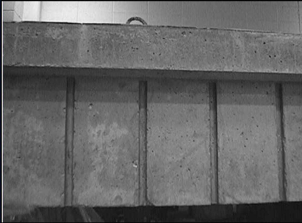
*Sawcut grooves for NSM reinforcement*
