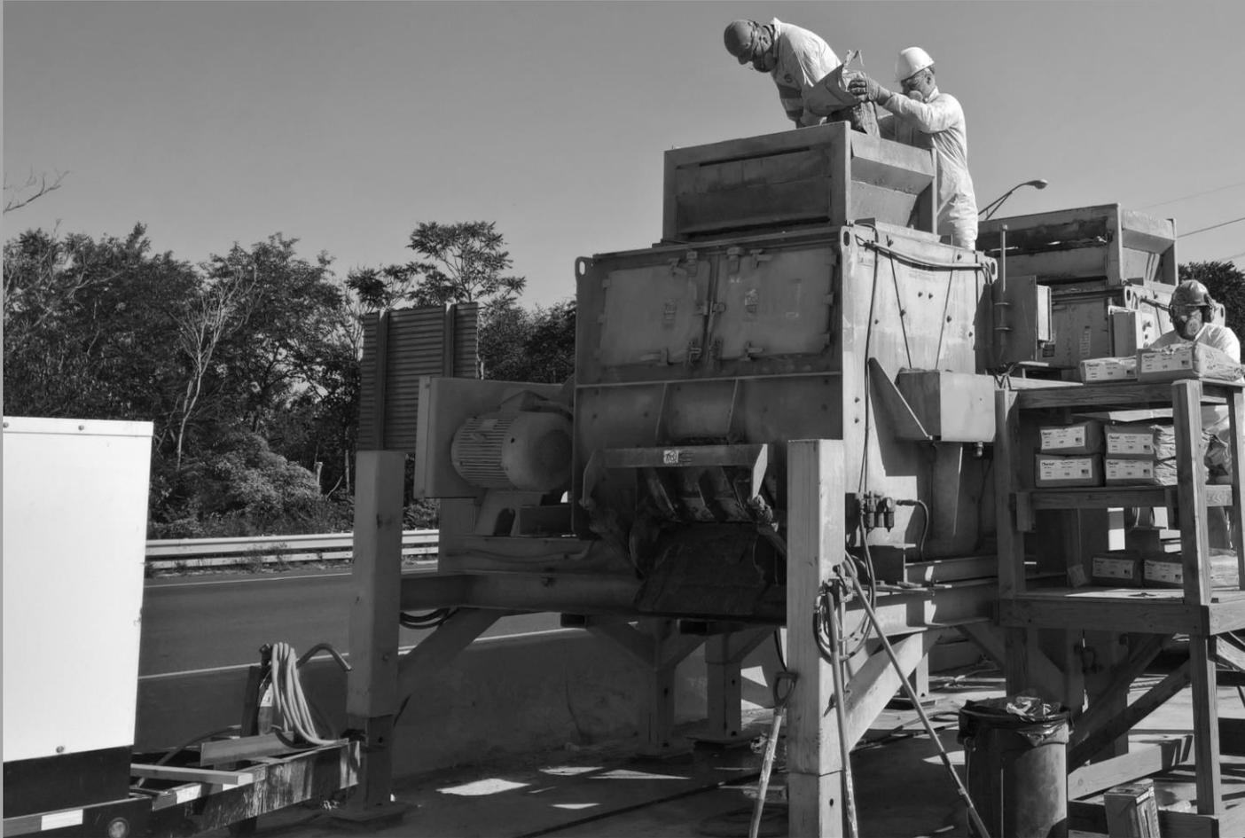
Horizontal shaft high-shear mixers
