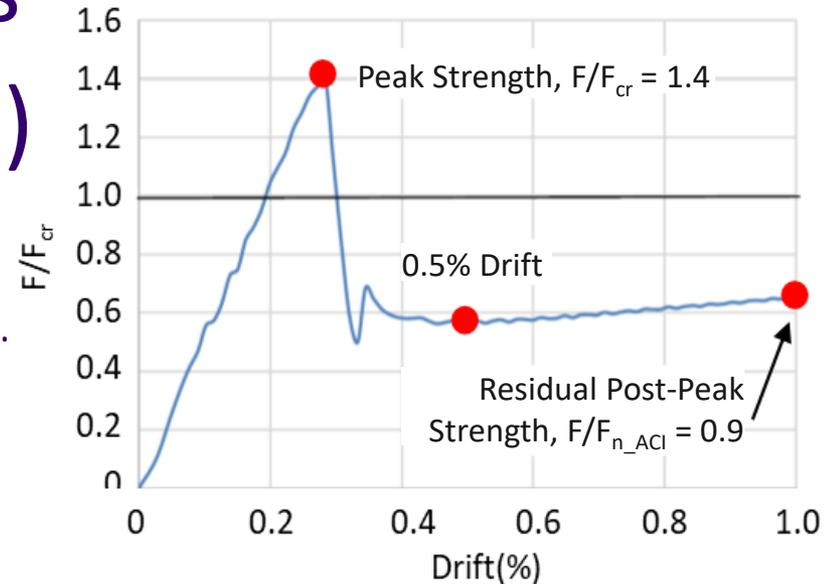
Concrete Damage Parameter
